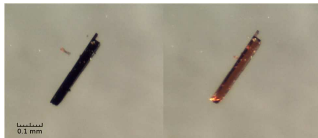
Figure 4. Light microscope image of SC-to-SC deoxygenation of [\{(bpbp)Co_2(O_2)_2\}_2(NH_2bdc)](NO_3)_4 \cdot 7H_2O , ( 2b ( NO_3 ) 4 · 7H_2O ) (left) to give [\{(bpbp)Co_2(NO_3)_2\}_2(NH_2bdc)](NO_3)_2 \cdot 2H_2O , 2b deoxy ( NO_3 ) 2 · 2H_2O (right). Transformation performed by heating for approximately 5 minutes on a regular hot-plate set to a temperature of 80 °C.
