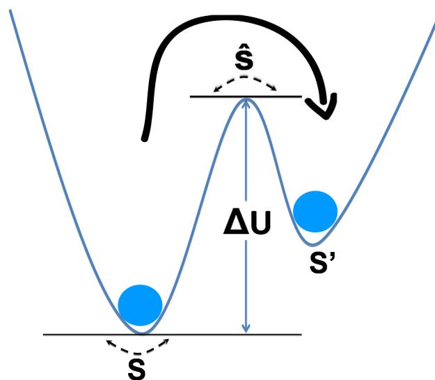
**Fig. 1** (Color online) The potential barrier  $\Delta U$  for calculating the transition state or Kramers' escaping rate. The basins of attractions are localized at  $S$  and  $S'$ .  $\hat{S}$  is the saddle point.
