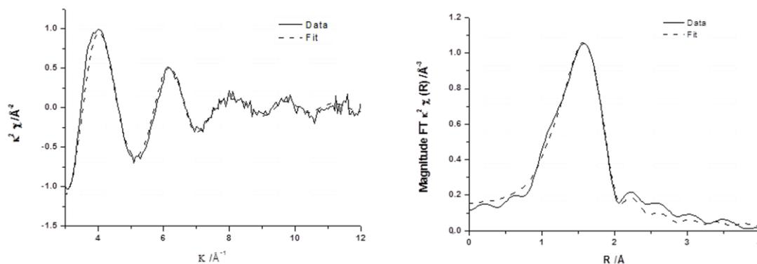
**Figure 7.**  $k^2$  experimental  $\chi$  data and fit (left) along with associated Fourier transform (right) for calcined 0.4wt%Fe-0.4wt%Cu/ZSM-5\_#13 prepared by CVI.
