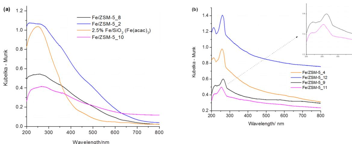
**Figure 2.** DR UV-vis absorbance spectra of various Fe/ZSM-5 and Fe/SiO<sub>2</sub> catalyst materials (a) heat treated at 550°C in air for 3h and (b) catalysts heat treated at 550°C in 5% H<sub>2</sub>/Ar for 3h.
