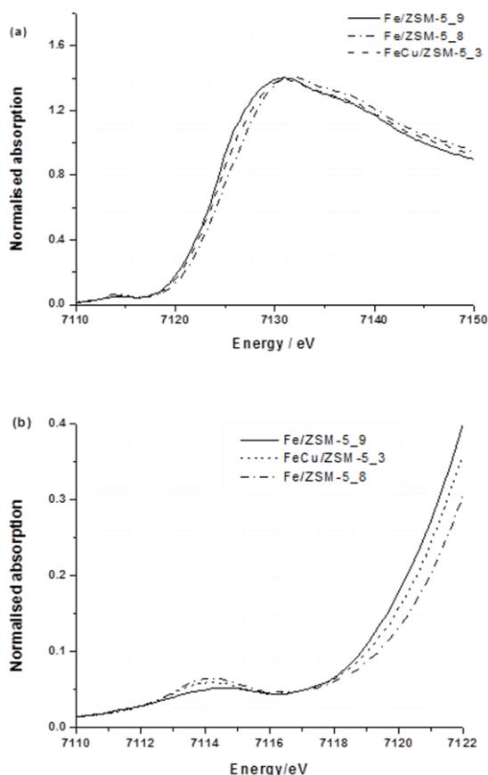
**Figure 6.** (a) XANES spectra and (b) Expanded pre-edge region of XANES spectra of 0.4wt%Fe-0.4wt%Cu/ZSM-5\_#13CVI samples.
