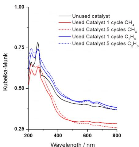
**Figure 9.** DR UV-vis spectra of 1.1wt%Fe/ZSM-5\_#4 employed in the oxidation of methane and ethane measured after one (1) and five (5) reaction cycles using  $\text{H}_2\text{O}_2$  as oxidant. Test conditions as in Figure 8, catalysts analysed at room temperature after air drying overnight.
