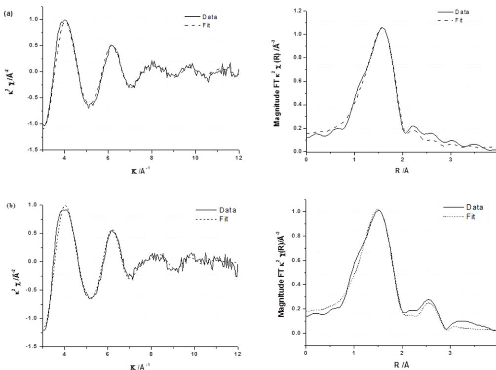
**Figure 5.**  $k^2$  experimental  $\chi$  data and fit (left) along with associated Fourier transform (right) for (a) 0.4wt%Fe/ZSM-5\_#9 and (b) 0.4wt%Fe/ZSM-5\_#8.
