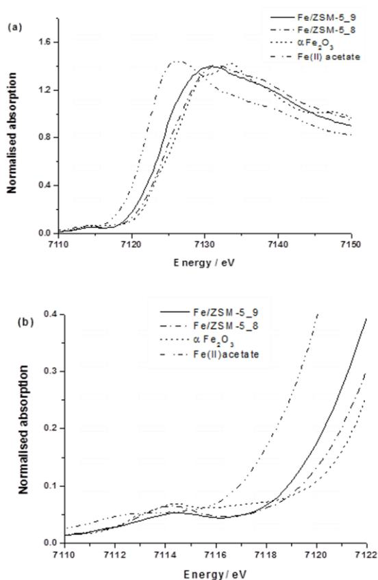
**Figure 4.** (a) XANES spectra and (b) expanded pre-edge region from various 0.4wt%Fe/ZSM-5(30) CVI samples.
