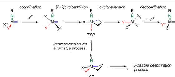
**Scheme 1.** Catalytic pathway proposed for  $d^0$  alkene metathesis
