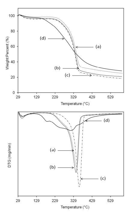
Fig 6: TGA and DTG curve of (a) CMF-NaClO<sub>2</sub>, (b) CMF-NaOH, (c) RNP-pulp and (d) nanocrystalline cellulose.
