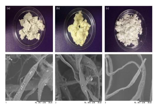
Fig. 2: Picture and scanning electron microscope image (a),(d) RNP as raw materials; (b) (e) Cellulose fiber after NaOH treatment; (c) (f) Cellulose fiber after NaClO<sub>2</sub> treatment.
