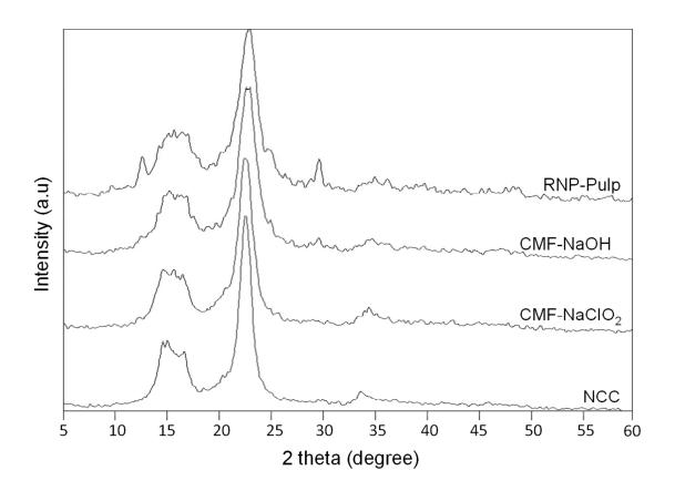
Fig 5: XRD pattern of RNP-pulp, CMF-NaOH, CMF-NaClO<sub>2</sub>, and NCC
