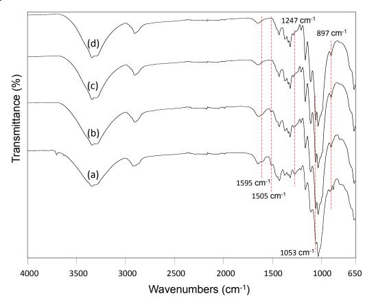
Fig 1: FTIR spectrum of recycled newspaper during isolation process: (a) RNP as raw material, (b) CMF-NaOH, (c) CMF-NaClO<sub>2</sub>, and (d) NCC after acid hydrolysis.
