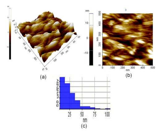
Fig 3: AFM image of NCC: (a) 3D view, (b) Height view, and (c) lateral size distribution.
