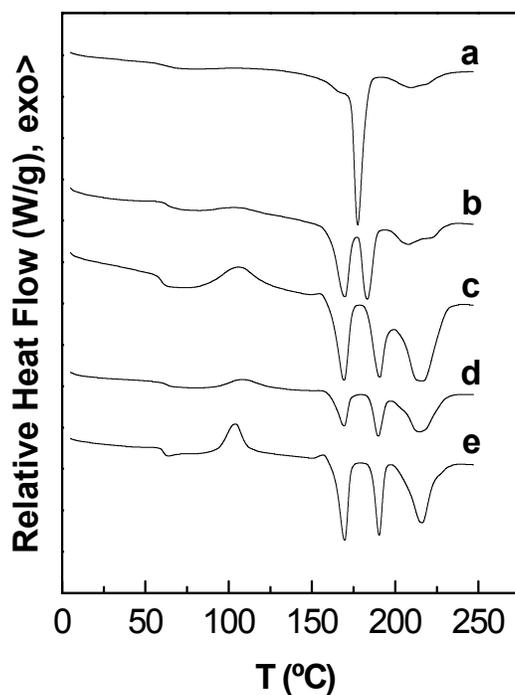
*Figure 6.* DSC curves of "as cast" B-5050 blends annealed at 180 °C for: (a) 30 min (b) 1h (c) 4h (d) 8h (e) 24 h.
