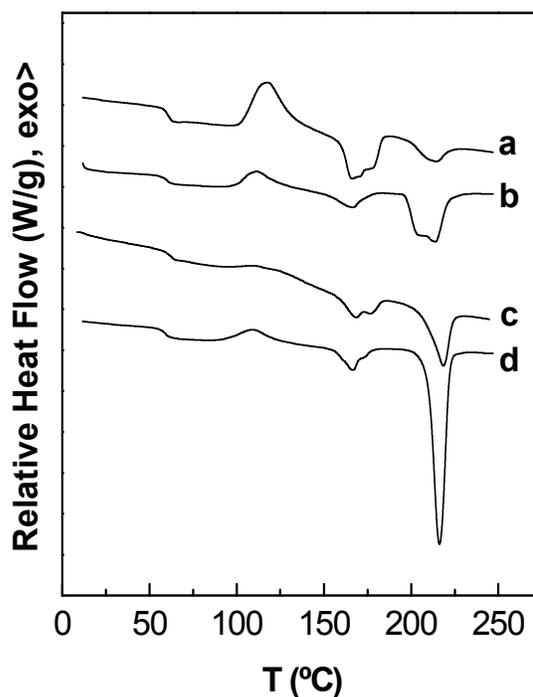
*Figure 7.* DSC curves of blends B-5050 after crystallization from melt with different isothermal treatments: (a) 190 °C for 1 h, (b) 190 °C for 1h after 130 °C for 10 min, (c) 190 °C for 24 h and (d) 190 °C for 24 h after 130 °C for 10 min.
