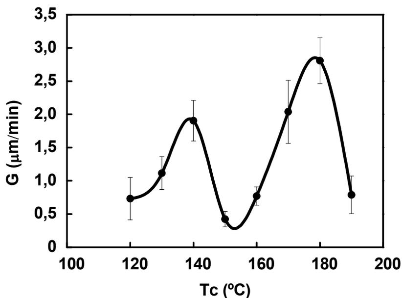
Figure 2. Radius growth rate of spherulites (G) of B-5050 blends as a function of crystallization temperature ( $T_c$ ).
