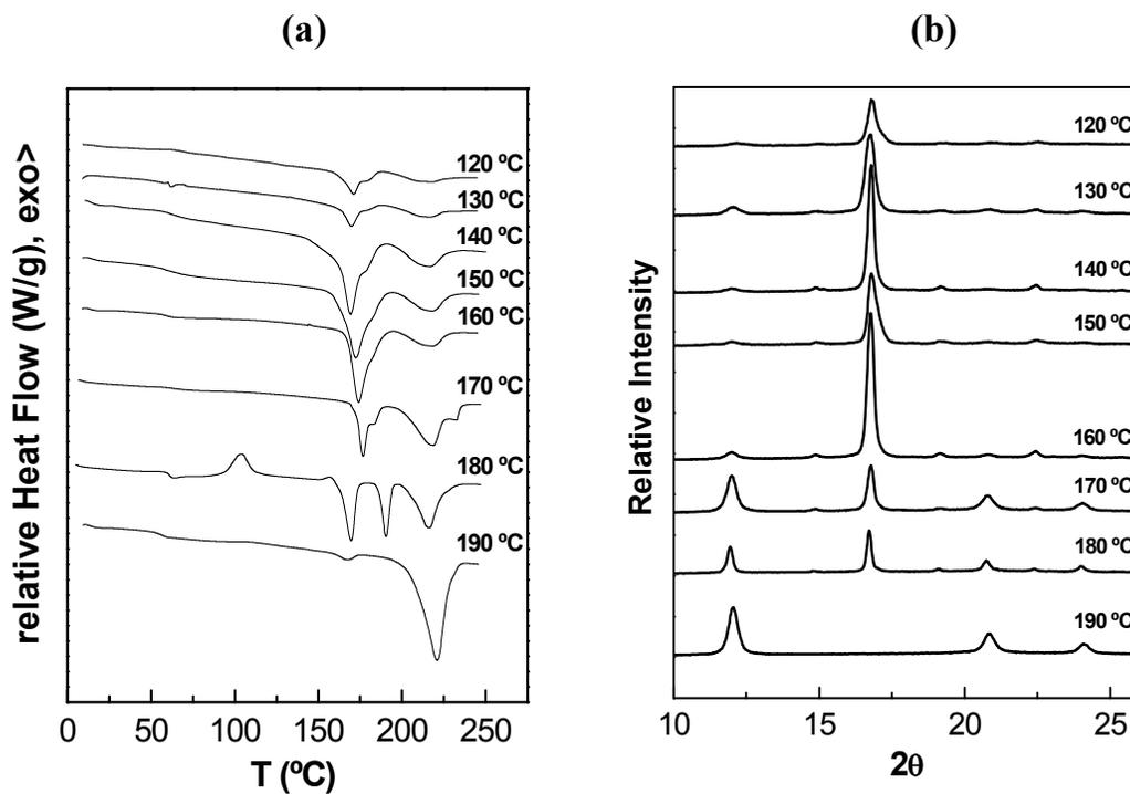
Figure 4. (a) DSC curves and (b) WAXD profiles of B-5050 blends annealed after “casting” at different crystallization temperatures for 24 h.
