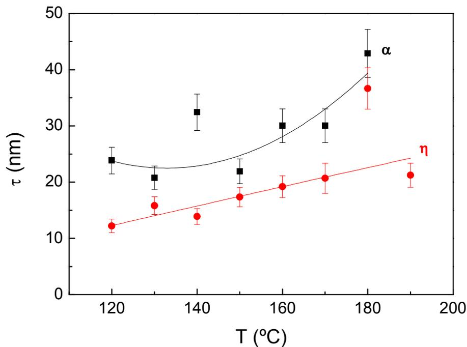
Figure 5. Evolution of crystalline domain size of B-5050 blends annealed after “casting” at different crystallization temperatures for 24 h.
