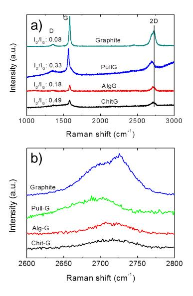
**Figure 7.** (a) Raman spectra of graphite, pull-G, alg-G, and chit-G; (b) detail of the 2D Raman band.
