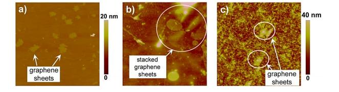
**Figure 6.** AFM height images  $(5 \times 5 \ \mu m^2)$  of (a) pull-G, (b) alg-G and (c) chit-G nanosheets deposited on mica substrates.
