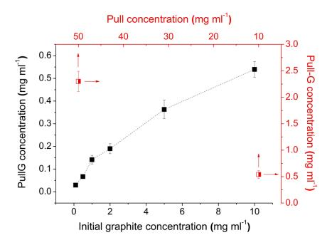
**Figure 1.** Effect of initial graphite concentration (full squared), and pullulan concentration (half squared) on the yield of graphene exfoliation (ultrasonication time 30 min).
