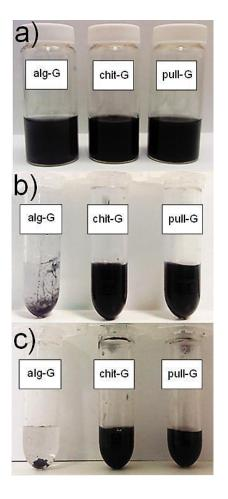
**Figure 3.** Digital images of freshly-prepared graphene (10 mg/ml) in alginate (50 mg/ml), chitosan (20 mg/ml), and pullulan (50 mg/ml) water dispersions after (a) 24 h; (b) 7 days; and (c) 6 months storage at room temperature.
