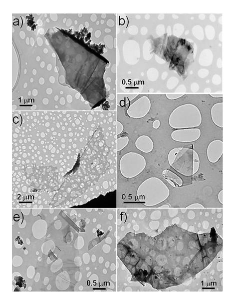
**Figure 2.** TEM images of pull-G for: (a) 10 min; (b) 20 min; (c) 30 min; (d) 60 min; (e) chit-G for 30 min; (f) alg-G for 30 min.
