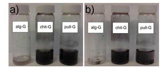
**Figure 5.** Digital images of redispersed alg-G (0.18 mg ml<sup>-1</sup>), chit-G (1 mg ml<sup>-1</sup>), and pull-G (1 mg ml<sup>-1</sup>) powders in water after (a) 24 h and (b) 7 days storage at room temperature.
