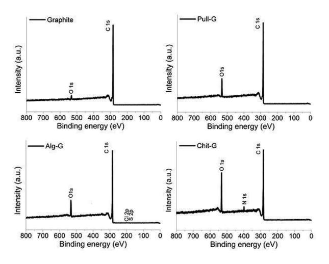
Figure 4. XPS survey spectra of pristine graphite powder, pull-G, alg-G, and chit-G.
