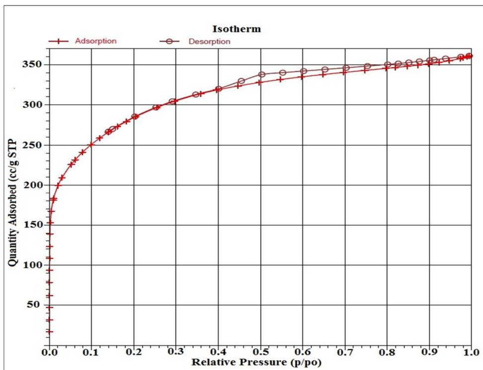
**Fig. 6. Nitrogen adsorption/desorption isotherm for the AC prepared at the optimum condition showing type I isotherm.**
