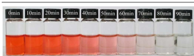
Fig. 10 The digital image of decolourization. (Initial dye concentration of ARG, 100 \text{ mg}\cdot\text{L}^{-1} ; current density, 50 \text{ mA}\cdot\text{cm}^{-2} ; concentration of supporting electrolyte ( \text{Na}_2\text{SO}_4 ), 0.1 \text{ M} )
