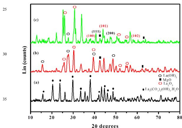
**Fig. 1** XRD pattern of (a) Mg-La-HT, (b) Mg-LaO (calcined at 650 °C) and (c) Ru/Mg-LaO (reduced at 450 °C).
