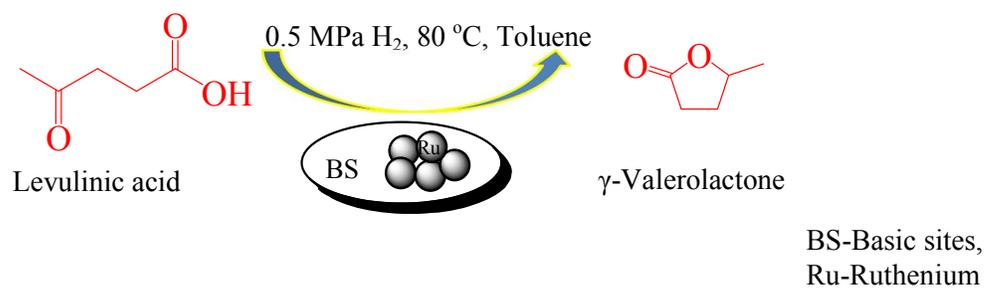
Ruthenium on a base support was developed for the conversion of biomass derived levulinic acid to  $\gamma$ -valerolactone at low temperature and pressure. This method provides general approach to  $\gamma$ -valerolactone synthesis which can replace ethanol in the petrol and in the production jet fuels.
