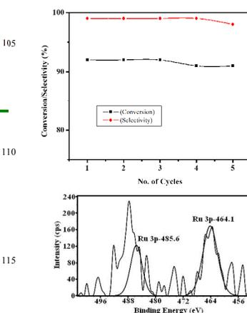
**Fig. 5** Recyclability studies on Ru/Mg-LaO for hydrogenation of LA at 80 °C, 0.5 MPa H<sub>2</sub> pressure.
