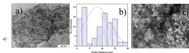
**Fig. 2** TEM images of a) reduced Ru/Mg-LaO (50 nm), b) particle size analysis and c) used Ru/Mg-LaO (200 nm)
