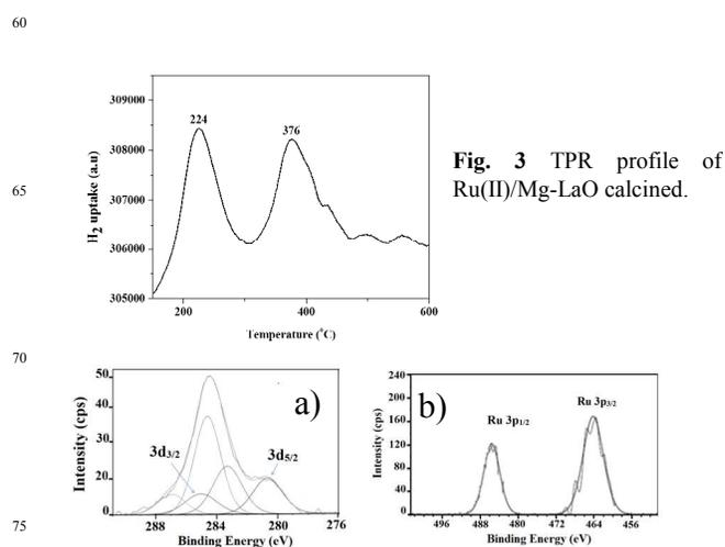
**Fig. 4** XPS spectra of Ru/Mg-LaO a) Ru 3d and b) Ru 3p.
