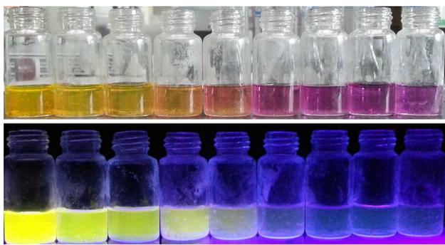
**Fig. 4** Photograph of solutions of 5  $\mu$ M BOPHY dye **3a** at pH 0, 1, 1.5, 2, 2.5, 3, 3.5, 4 and 7 in CH<sub>3</sub>CN/H<sub>2</sub>O (1:1, v/v) under normal room illumination (upper row) and under UV irradiation (bottom row), respectively.
