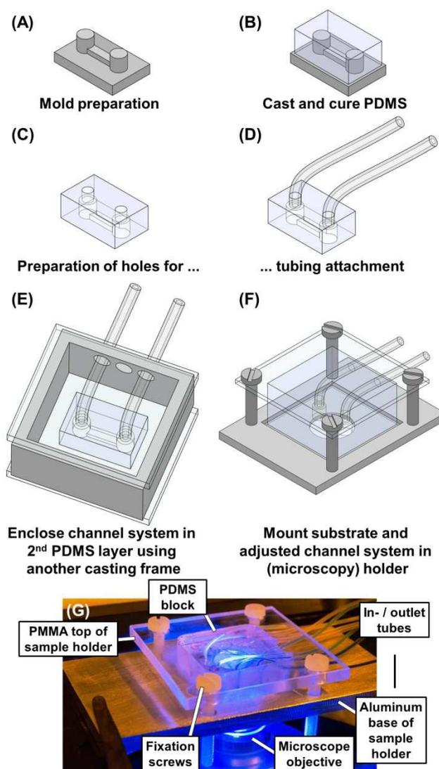
**Fig. 1** Schematic illustration of the production steps during the PDMS setup fabrication. (A-F) and a photograph of one finished and assembled device (G).
