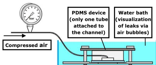
**Fig. 2** Schematic drawing of the leakage test arrangement. Compressed air is pushed pressure controlled into a PDMS device with only one attached tube. Having the whole set-up inside a water bath allows checking for air bubbles indicating a leak.
