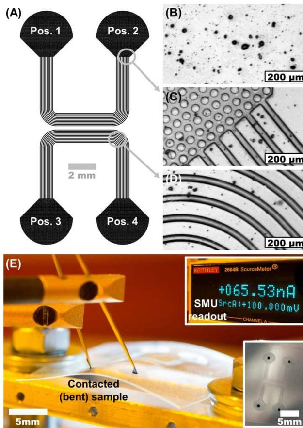
**Fig. 3** Layout of the channel design for printing PEDOT:PSS based flexible electronics (A). Optical microscopy images of the printer foil which was utilized as substrate before any polymer deposition (B), of the in- / outlet area (C) and one curved line section (D) after PEDOT:PSS printing. Photograph of the conductivity measurement arrangement and in the insets the simultaneously displayed data on the SMU readout and a photograph of the whole circuit, respectively (E).
