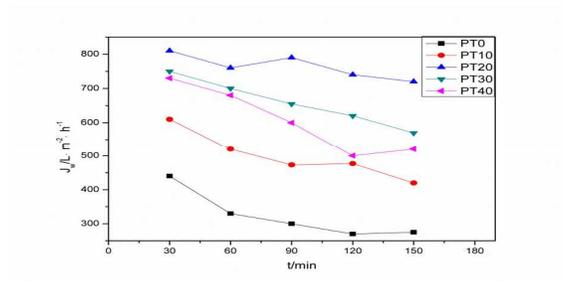
PVDF/SiO<sub>2</sub> membranes by sol-gel were characterized and ultrafiltration performance of fennel oil in water extract through them was effectively improved.
