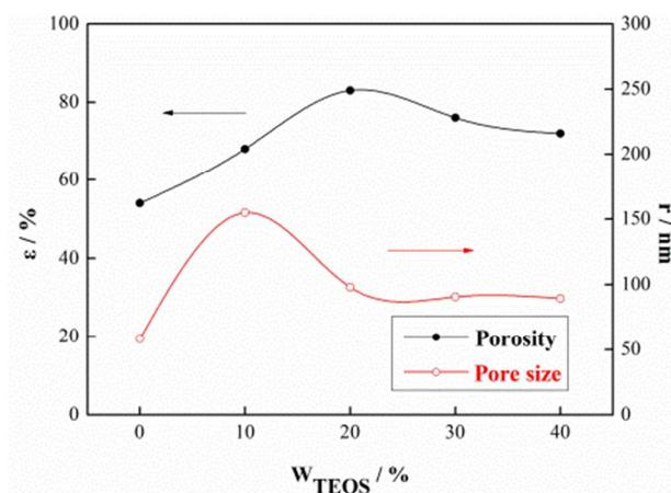
**Fig. 8** The effects of TEOS content on porosity and pore size of membranes
