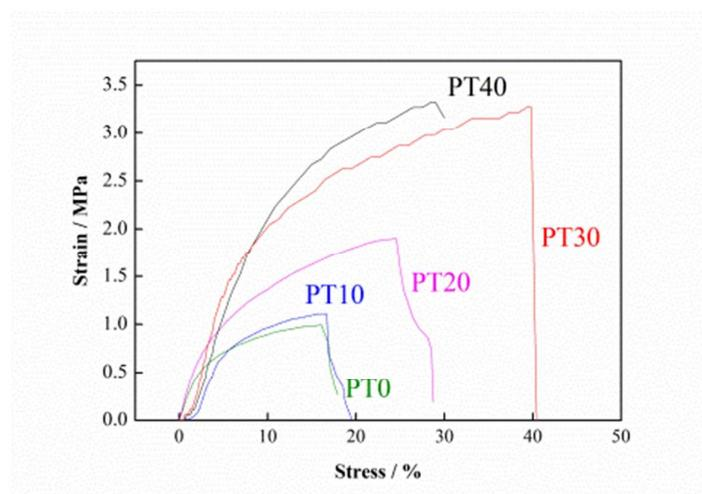
**Fig.5 Stress-strain curves of unfilled and hybrid membranes**
