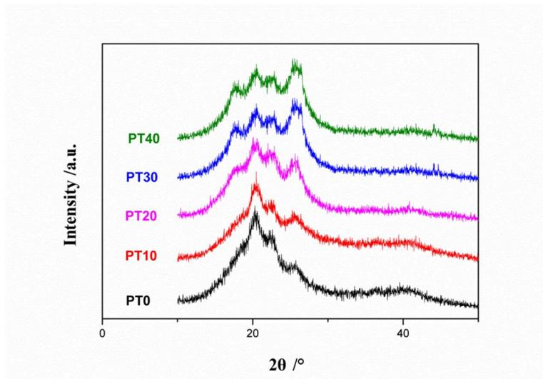
Fig. 2 XRD patterns of unfilled and hybrid membranes
