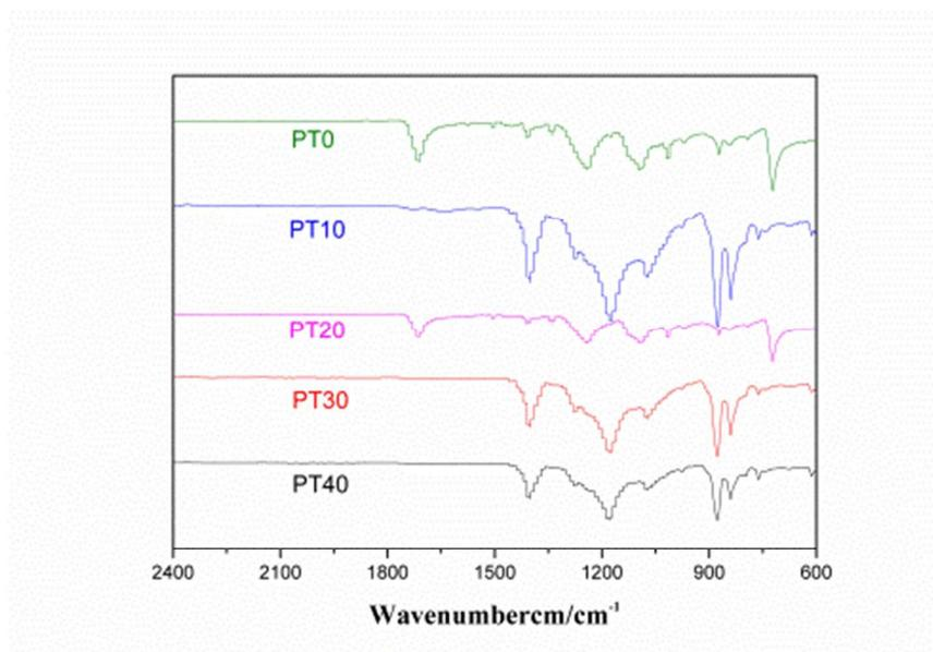
Fig. 1 FTIR spectra of unfilled and hybrid membranes
