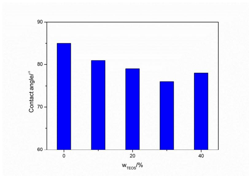
**Fig. 7** The effects of TEOS content on the water contact angle values of membranes
