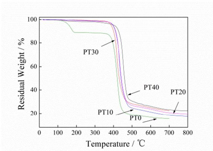
**Fig.4 TGA curves of unfilled and hybrid membranes**
