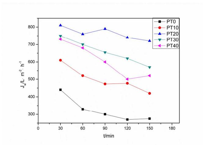
Fig. 12 The dependence of water flux containing fennel oil through membranes on time
