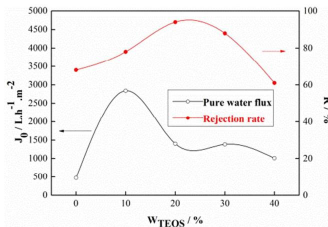
**Fig. 9** The effects of TEOS content on pure water flux and rejection rate of membranes
