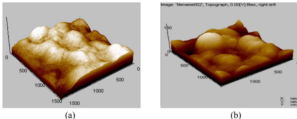
Fig. 6 AFM three-dimensional surface images of PT0 (a) and PT20 (b) membranes
