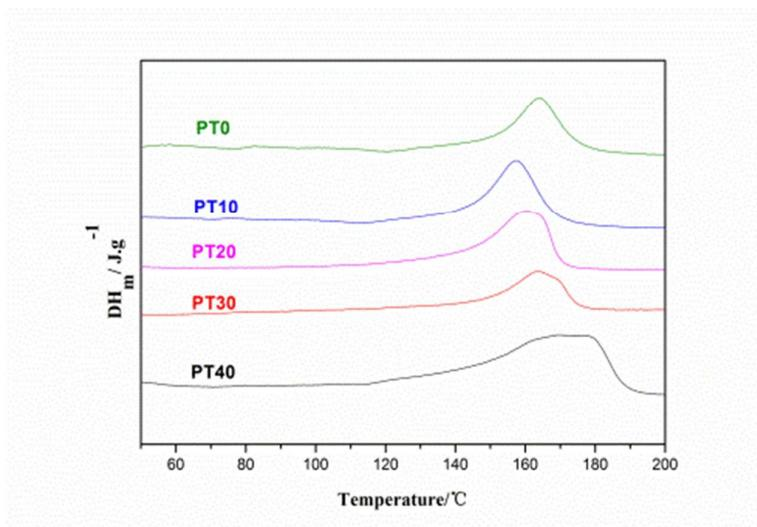
**Fig. 3 DSC thermograms of unfilled and hybrid membranes**
