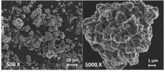
Fig. 3 SEM micrographs of a used catalyst.
