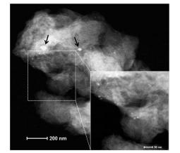
Fig. 4 STEM micrograph of the catalyst used in six reaction cycles at 40 W during 5 min, showing large Pd nanoparticles (black arrows), together with smaller ones.
