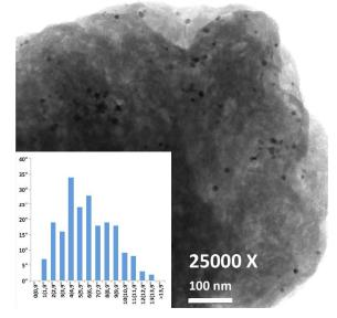
Fig. 1 Size distribution of the supported Pd nanoparticles in the fresh catalysts.
