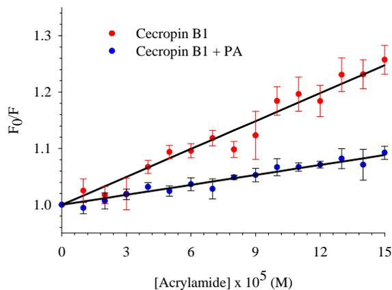
**Fig. 2** Stern-Volmer plots for the fluorescence quenching of tryptophan in cecropin B1 by acrylamide in the absence and presence of the PA membrane. The concentration of PA and cecropin B1 was 0.05 mM (1:1 molar ratio).  $\lambda_{\text{ex}} = 295$  nm.
