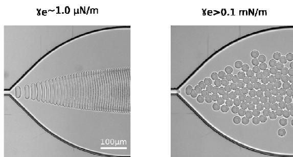
A microfluidic platform was used to generate monodisperse oil-in-water emulsion, whose final interfacial tension was actively lowered to ultra-low values.
