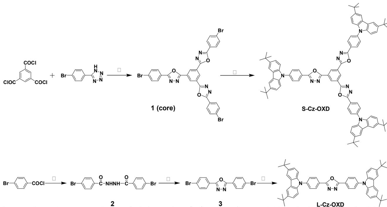
**Scheme 1** Synthesis route to S-Cz-OXD and L-Cz-OXD. i) anhydrous pyridine; reflux for 24 hours. ii) 3,6-Di-tert-butyl-9H-carbazole, CuI, K<sub>2</sub>CO<sub>3</sub>, 1,3-dimethyl-3,4,5,6-tetrahydro-2(1H)-pyrimidinone (DMPU), and 18-crown-6; 170 °C for 48 hours. iii) H<sub>2</sub>NNH<sub>2</sub>·H<sub>2</sub>O, Et<sub>3</sub>N, CH<sub>2</sub>Cl<sub>2</sub>; 40 °C for 2 hours. iv) SOCl<sub>2</sub>, toluene; reflux for 12 hours.
