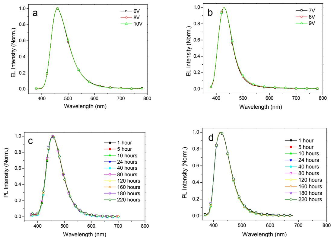
**Figure 4.** Normalized EL spectra of devices based on (a) S-Cz-OXD and (b) L-Cz-OXD at different applied voltages, and PL spectra of (c) S-Cz-OXD and (d) L-Cz-OXD during heating process at 150 °C in ambient air
