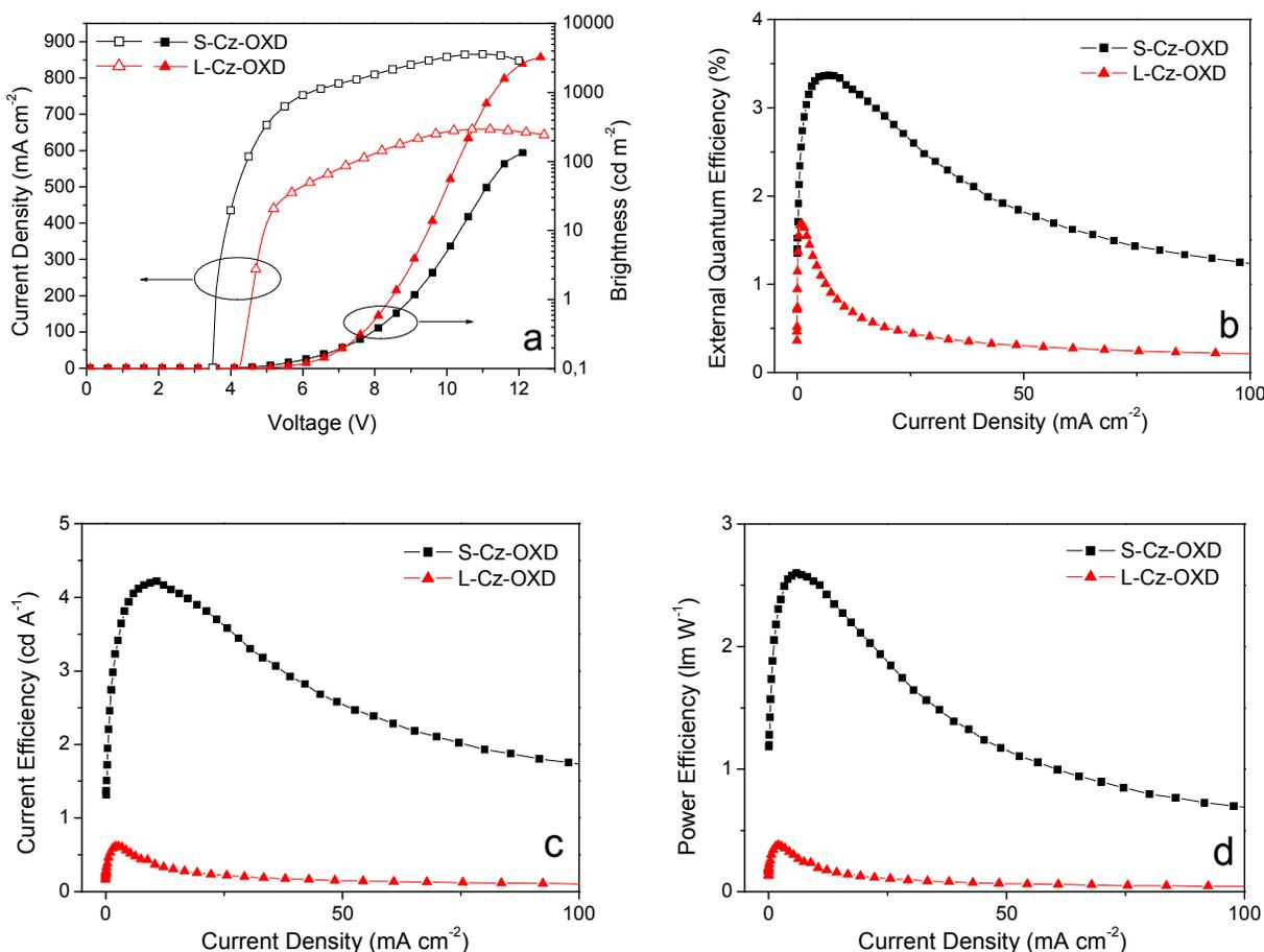
**Figure 5.**(a) Current density–voltage and brightness–voltage spectra of devices; (b) Current efficiency versus current density of devices; (c) Power efficiency versus current density of devices; (d) External quantum efficiency versus current density of devices.
