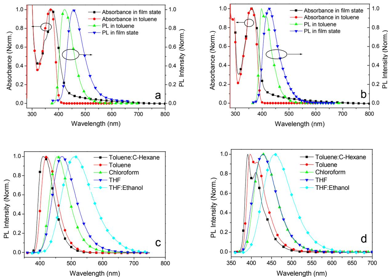
**Figure 1.** Absorption and PL spectra of (a) S-Cz-OXD and (b) L-Cz-OXD in dilute toluene solution and film state, and PL spectra of (c) S-Cz-OXD and (d) L-Cz-OXD in various solvents.
