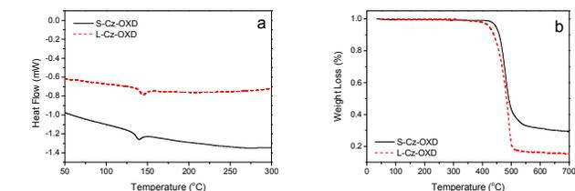
**Figure 3.** (a) DSC traces and (b) TGA thermogram of S-Cz-OXD and L-Cz-OXD
