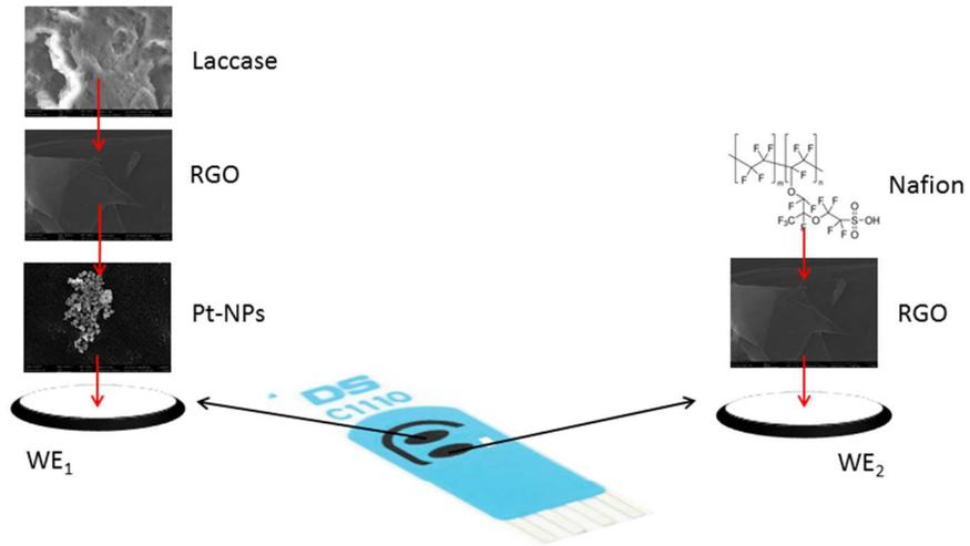
Schematic representation of the developed disposable dual sensor array.
