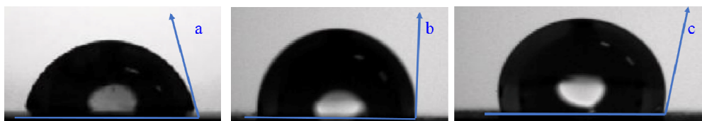
Fig. 7 Sessile water drop images on: (a) a bare copper surface, (b) a copper surface covered with 0.15\text{mmol L}^{-1} AND, and (c) a copper surface covered with 0.15\text{mmol L}^{-1} DSM.
