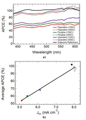
Fig. 8 a) APCE of different  $TiO_2$  electrodes heat treated at 150°C and 450°C; b) Plot of average APCE vs. Jsc of  $TiO_2$  electrode.
