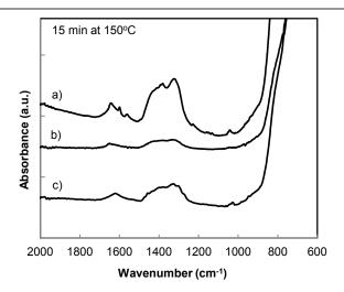
Fig. 3 FTIR spectra of TiO<sub>2</sub> films synthesised using: a) quinoline, b) pyridine and c) piperidine after heat treated at 150°C for 15 min.
