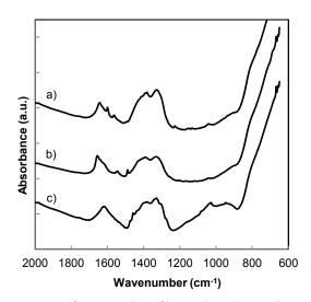
Fig. 2 FTIR spectra of as-prepared TiO<sub>2</sub> films synthesised using: a) quinoline, b) pyridine and c) piperidine.
