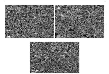
Fig. 5 SEM images of a) piperidine, b) pyridine and c) quinoline-based  $TiO_2$  films after 15 minutes at 150°C
