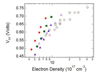
Fig. 9 Open-circuit voltage as a function of electron density in the TiO<sub>2</sub> film. Piperidine:  $\bullet$  - 150°C,  $\bigcirc$  - 450°C; Pyridine:  $\bullet$  - 150°C,  $\bigcirc$  - 450°C; Quinoline:  $\blacktriangle$  - 150°C,  $\triangle$  - 450°C; and  $\diamondsuit$  - Solaronix reference.
