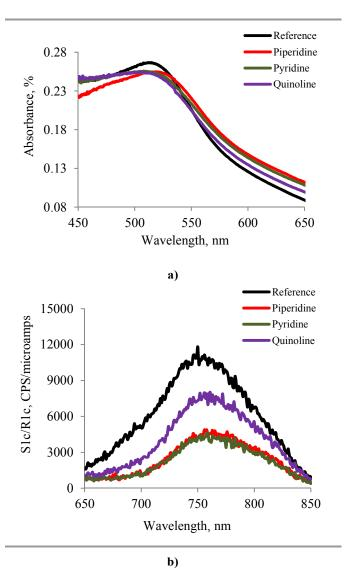
Fig. 10 a) Absorption of N719 and b) emission spectra of N719 excited at 520nm for  $Al_2O_3$  films prepared with different binders.
