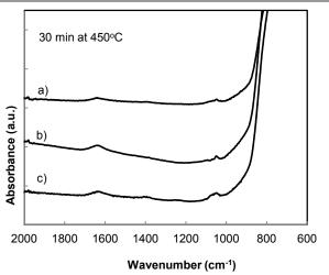
Fig. 4 FTIR spectra of TiO<sub>2</sub> films synthesised using: a) quinoline, b) pyridine and c) piperidine after heat treated at 450°C for 30 min.
