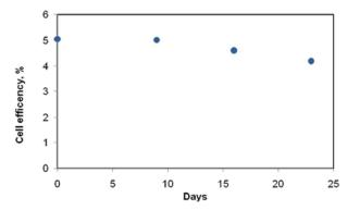
Fig. 6 Cell efficiency averaged over 4 cells produced from the quinoline based paste monitored over 25 days.
