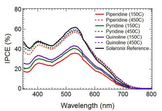
Fig. 7 IPCE of different  $TiO_2$  electrodes heat treated at  $150^{\circ}C$  and  $450^{\circ}C$ .
