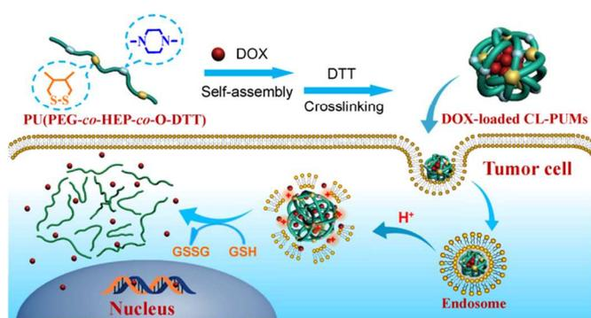
**Scheme 1.** Schematic illustration for the formation of DOX-loaded CL-PUMs as well as the structural transitions of the nano-carriers in response to acidic micro-environment and GSH.
