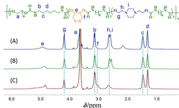
**Figure 1.** <sup>1</sup>H NMR spectra of PU(PEG-co-HEP-co-O-DTT)-1 (A), -2 (B) and -3 (C) in CDCl<sub>3</sub>.
