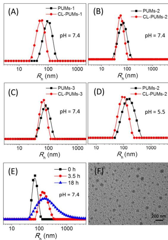
**Figure 3.** The hydrodynamic radii ( $R_h$ ) of PUMs-1 and CL-PUMs-1 (A), PUMs-2 and CL-PUMs-2 (B), PUMs-3 and CL-PUMs-3 (C) at pH 7.4; PUMs-2 and CL-PUMs-2 (D) at pH 5.5; change in  $R_h$  of CL-PUMs-2 after addition of 10 mM GSH at pH 7.4 (E); TEM image taken after drying of the CL-PUMs-2 aqueous solution (F).
