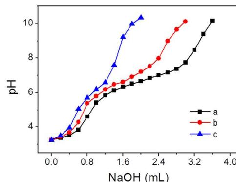
**Figure 2.** Acid-base titration curve of the acidified solution of PU(PEG-co-HEP-co-O-DTT)-1 (a), -2 (b) and -3 (c) titrated with 0.1 N NaOH.
