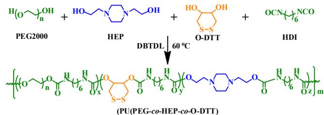
**Scheme 2.** Synthesis route of PU(PEG-co-HEP-co-O-DTT) multiblock copolymers.
