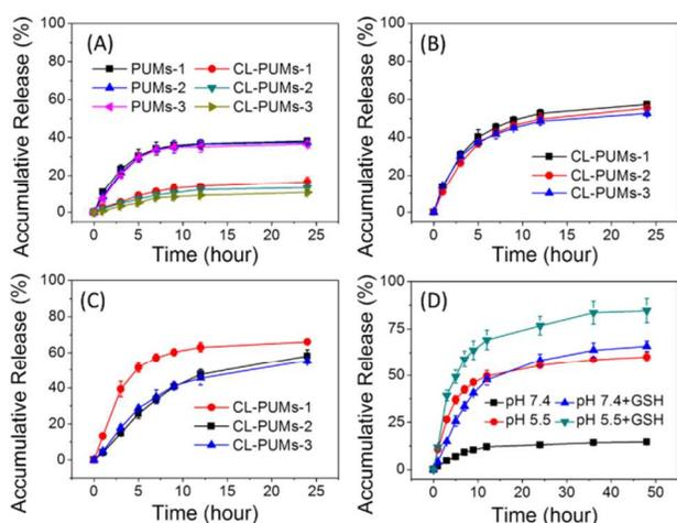
**Figure 4.** The drug release behaviors of DOX-loaded PUMs and CL-PUMs in PBS at different conditions. (A) DOX-loaded PUMs and CL-PUMs at pH 7.4 without GSH; (B) DOX-loaded CL-PUMs at pH 5.5 without GSH; (C) DOX-loaded CL-PUMs at pH 7.4 with 10 mM GSH; (D) DOX-loaded CL-PUMs-2 under different stimuli. Data are presented as the average  $\pm$  standard deviation ( $n = 3$ ).
