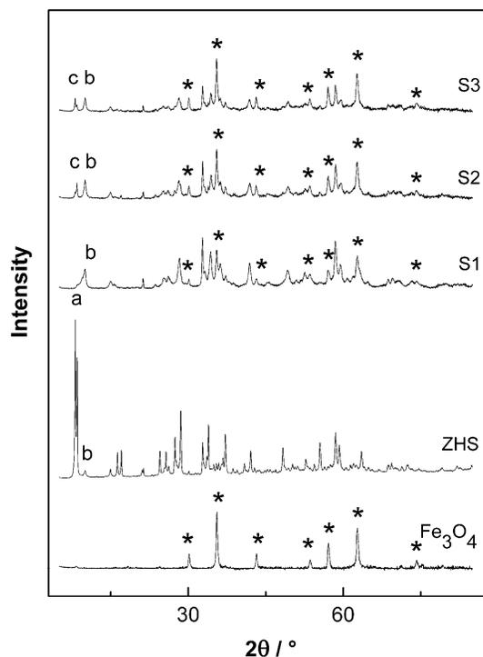
Fig. 2: XRD patterns of the reactants and products of the synthesis, when samples S1, S2 and S3 contain 50 mg, 100 mg and 150 mg of Fe<sub>3</sub>O<sub>4</sub> for the synthesis.
