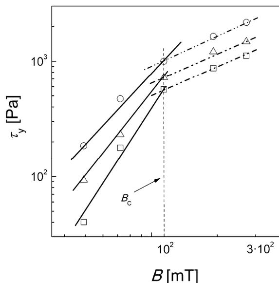
Fig. 10: Dependence of the yield stress,  $\tau_y$ , on the magnetic flux density,  $B$ , for particle silicone oil suspensions where ( $\square$ ) 80 wt.% of bare CI, ( $\triangle$ ) 80 wt.% of bare CI together with 1 wt.% of sheet-like additive S3 and ( $\circ$ ) 80 wt.% of bare CI together with 5 wt.% of sheet-like additive S3.
