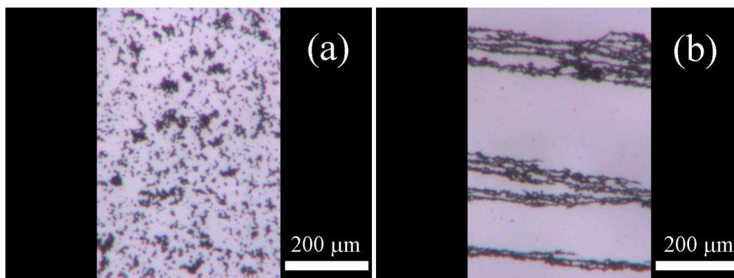
Fig. 8: Microscopic observation of the suspension containing 20 wt. % of bare CI particles and corresponding amount of additive S3 (1 wt. %) (a) in the absence of the magnetic field and (b) in the presence of the magnetic field of 120 mT.
