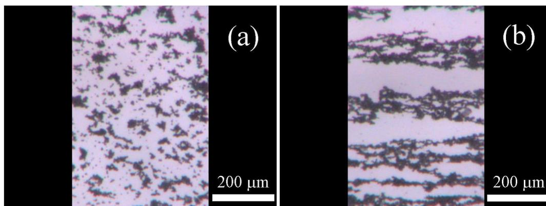
Fig. 9: Microscopic observation of the suspension containing 20 wt. % of bare CI particles and corresponding amount of additive S3 (5 wt. %) (a) in the absence of the magnetic field and (b) in the presence of the magnetic field of 120 mT.
