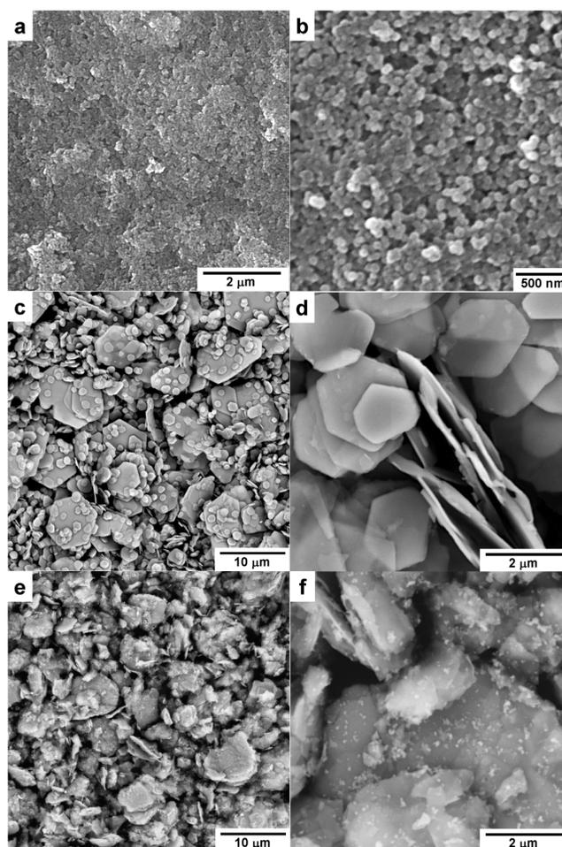
Fig. 3: SEM images of  $\text{Fe}_3\text{O}_4$  nanoparticles (a, b), sample S2 (c, d) and sample S3 (e, f) at various magnifications.
