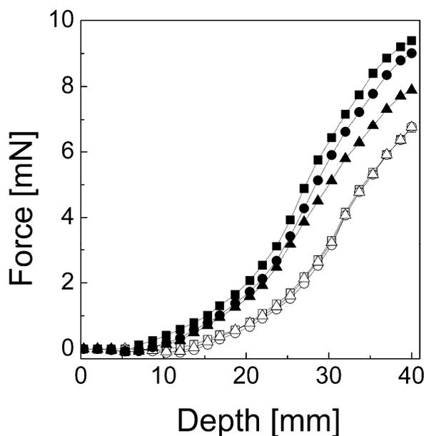
Fig. 5: Dependence of the penetration force against depth for suspensions including 80 wt. % of the bare CI particles (■, □), 80 wt. % of the bare CI particles together with 1 wt. % of sheet-like additive S3 (●, ○) and 80 wt. % of the bare CI particles together with 5 wt. % of sheet-like additive S3 (▲, △) in silicone oil for just prepared suspensions (open symbols) and measured after 7 days (solid symbols).
