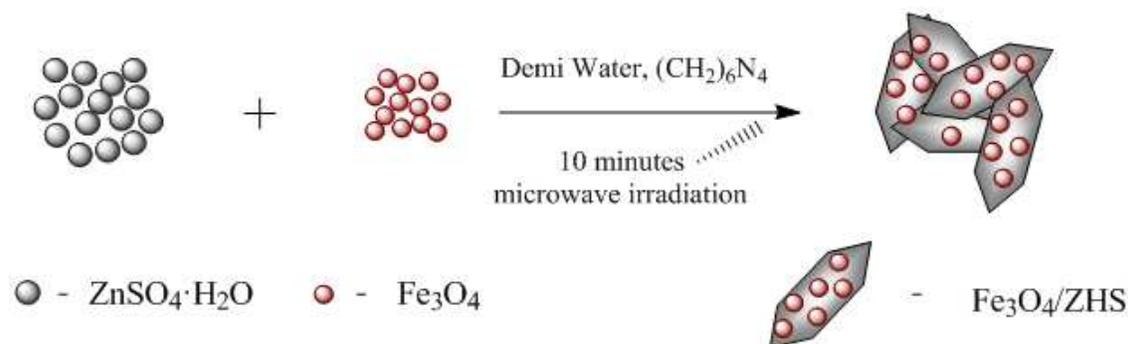
Fig. 1: Schematic illustration of  $\text{Fe}_3\text{O}_4/\text{ZHS}$  hybrid composite sheets synthesis procedure.
