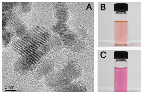
Figure 1. The TEM images of nano-ceria (A); Appearance of the DIF suspension (B) and the suspension of DIF-coated nano-ceria (C).
