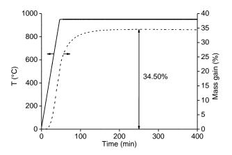
Fig. 2 Thermogravimetric analysis of the magnet powder <400  $\mu$ m. The NdFeB magnet powder was first heated to 950 °C (heating rate: 20°C min<sup>-1</sup>) and kept at this temperature for another 6 h. The temperature of the furnace is given by the solid line and the mass gain (%) by the dashed line.
