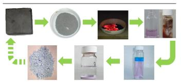
A recycling process was developed in which only oxalic acid is consumed to remove and separate the rare-earth metals from NdFeB magnets.
