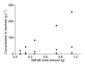
Fig. 9 Concentration of neodymium (■), dysprosium (▼), cobalt (o) and iron (x) in the leachate as a function of the amount of magnet oxide powder involved in leaching with 1 mL of aqueous phase. The n(HCl)/n(Ln) ratio was 3.5 and the pH
