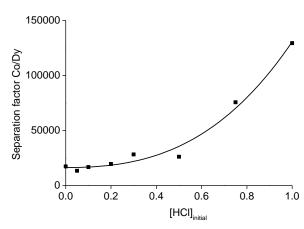
Fig. 12 The separation factors  $\alpha_{\text{Co,Dy}}$  between cobalt and dysprosium as a function of the initial HCl concentration of the aqueous phase. The aqueous phase contains 3.0 g L<sup>-1</sup> cobalt, 25 g L<sup>-1</sup> Dy and 3.5 NH<sub>4</sub>Cl. The organic phase was trihexyl(tetradecyl)phosphonium chloride mixed with the aqueous phase in a volume ratio of 1.
