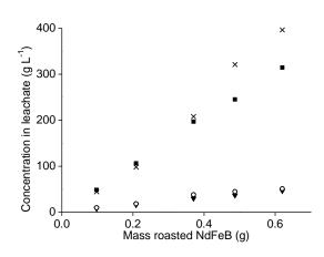
Fig. 11 Concentration of neodymium chloride ( $\blacksquare$ ), dysprosium chloride ( $\blacktriangledown$ ), cobalt chloride (o), and iron(II,III) chloride (x) as a function of the amount of magnet oxide powder involved in leaching with 1 mL of aqueous phase. The n(HCl)/n(Ln) value was 10 and the pH after the extraction between 0.42 and - 0.56. Relative standard deviation < 4.2%.
