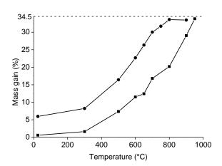
Fig. 3 Mass gain (%) of the <400  $\mu$ m ( $\blacksquare$ ) and <80  $\mu$ m ( $\bullet$ ) NdFeB magnet powder as a function of the temperature at which it was held for 1h. The dashed line is drawn at 34.5%, which is the maximum mass gain determined with TGA.
