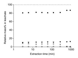
Fig. 8 Relative mass percentages of neodymium ( $\blacksquare$ ), dysprosium ( $\blacktriangledown$ ), cobalt (o) and iron (x) in the leachate as a function of extraction time for 0.1 gram or roasted NdFeB magnet in 1 mL of a diluted HCl solution with a n(HCl)/n(Ln) ratio of 3.5.
