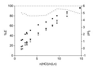
Fig. 7 Percentage extraction (%E) of neodymium ( $\blacksquare$ ), dysprosium ( $\blacktriangledown$ ), cobalt (o) and iron (x) as a function of the initial HCl leaching concentration for NdFeB magnet powder which was not roasted. The dashed line presents the measured
