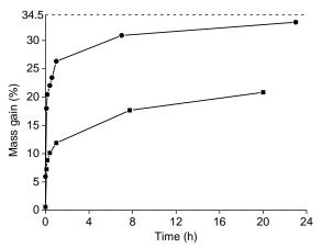
Fig. 4 Mass gain (%) of the <400  $\mu$ m ( $\blacksquare$ ) and <80  $\mu$ m ( $\bullet$ ) NdFeB magnet powder as a function of the roasting time at a temperature of 650 °C. The dashed line is drawn at 34.5%, which is the maximum mass gain determined with TGA.
