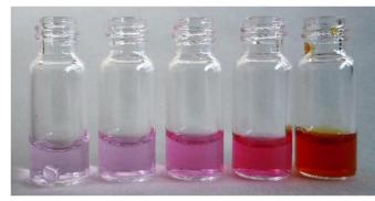
Fig 10. Color of the leachate when the amount of NdFeB magnet oxide powder, dissolved in 1 mL of diluted HCl and at constants n(HCl)/n(Ln) ratio of 3.5, was increased from left to right. The purple colour is characteristic for neodymium and the orange colour is due to a small amount of dissolved iron.
