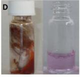
Fig. 1 (A) The NdFeB magnet before crushing and milling, (B) NdFeB powder (<400  $\mu$ m) before roasting, (C) roasting and powder fire at high temperatures and (D) the leachate colored pink-violet by neodymium (right) and the remaining orange/brown iron(III) hydroxide precipitate (left).
