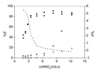
Fig. 6 Extraction percentages (%E) of neodymium ( $\blacksquare$ ), dysprosium ( $\blacksquare$ ), cobalt (O) and iron ( $\times$ ) as a function of the molar ratio of HNO $_3$  over the rare earths present in the roasted NdFeB magnet powder. The dashed line shows the measured final pH values (pH $_f$ ) after the leaching experiments. Relative standard deviation < 6.9%
