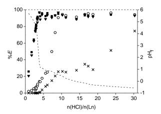
Fig. 5 Extraction percentages (%E) of neodymium ( $\blacksquare$ ), dysprosium ( $\blacksquare$ ), cobalt (O) and iron (x) as a function of the molar ratio of HCl over the rare earths present in the roasted NdFeB magnet powder (15 h at 80 °C) The dashed line shows the measured final pH values (pH<sub>f</sub>) after the leaching experiments. Relative standard deviation < 6.9%.
