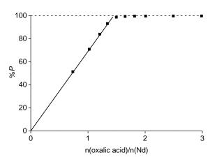
Fig. 13 Precipitation percentage (%P) as a function of the molar ratio of oxalic acid added to the solution over neodymium present in the aqueous phase n(oxalic acid)/n(Nd). The aqueous phase contained of 26.7 g L $^{-1}$  neodymium and 3.5 M NH $_4$ Cl.
