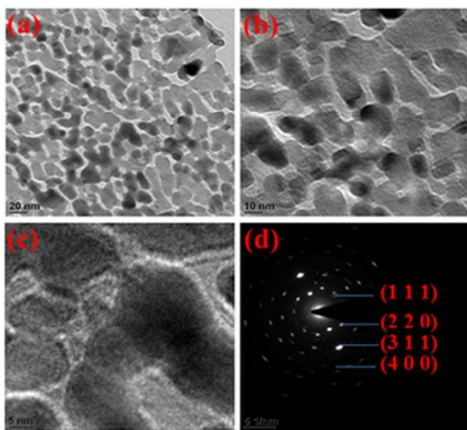
Figure 3. (a-e) HRTEM images of  $\text{Co}_3\text{O}_4$  nanoflower and (f) the corresponding SAED pattern.
