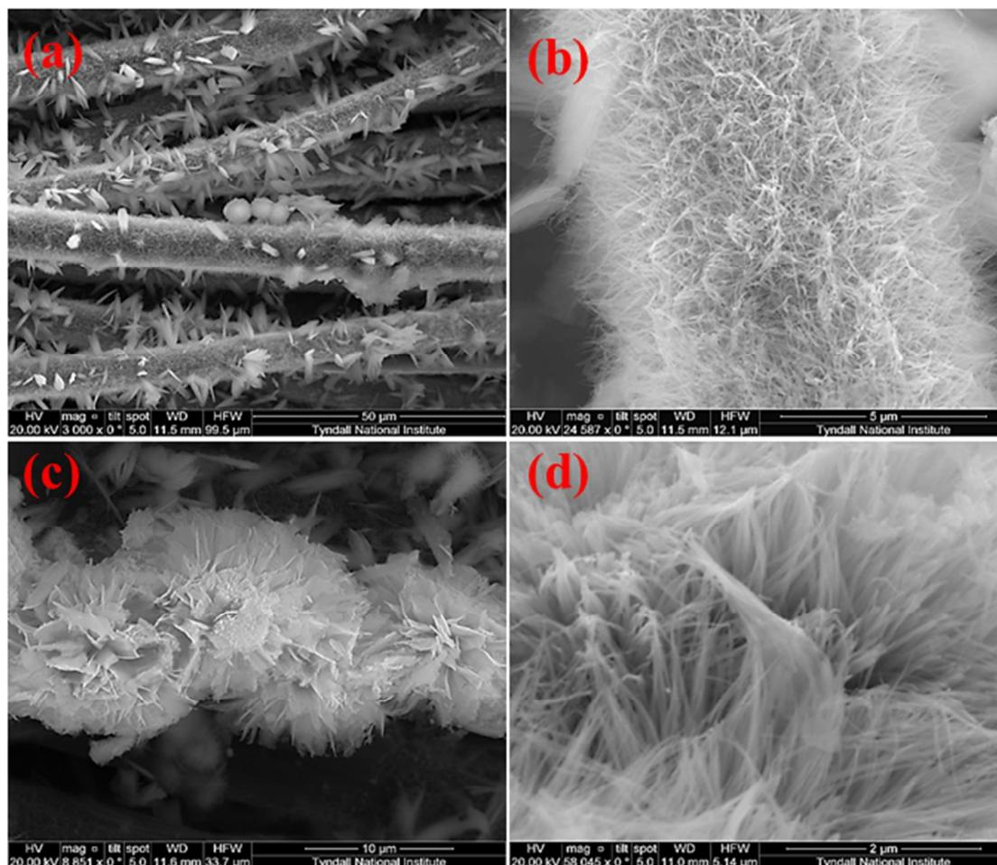
Figure 2. (a-d) HRSEM images of  $\text{Co}_3\text{O}_4$  nanowire/nanoflower on CFC at different magnifications.
