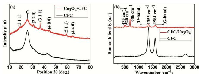
Figure 1. (a) XRD patterns and (b) Raman spectra of CFC (Black) and  $\text{Co}_3\text{O}_4/\text{CFC}$  (Red).
