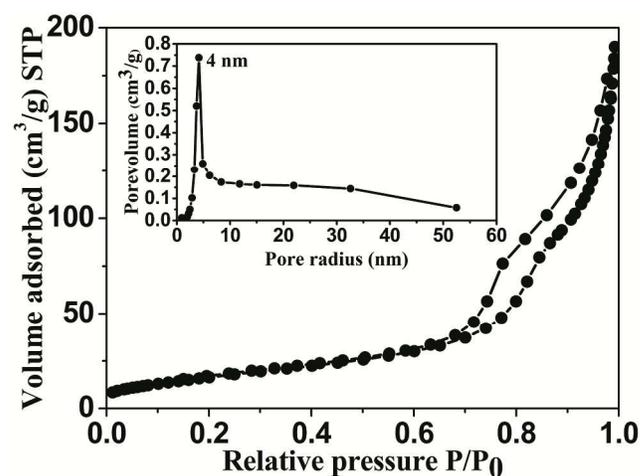
Figure 4.  $\text{N}_2$  adsorption and desorption curve of  $\text{Co}_3\text{O}_4$  nanostructure and the corresponding pore size distribution (inset).
