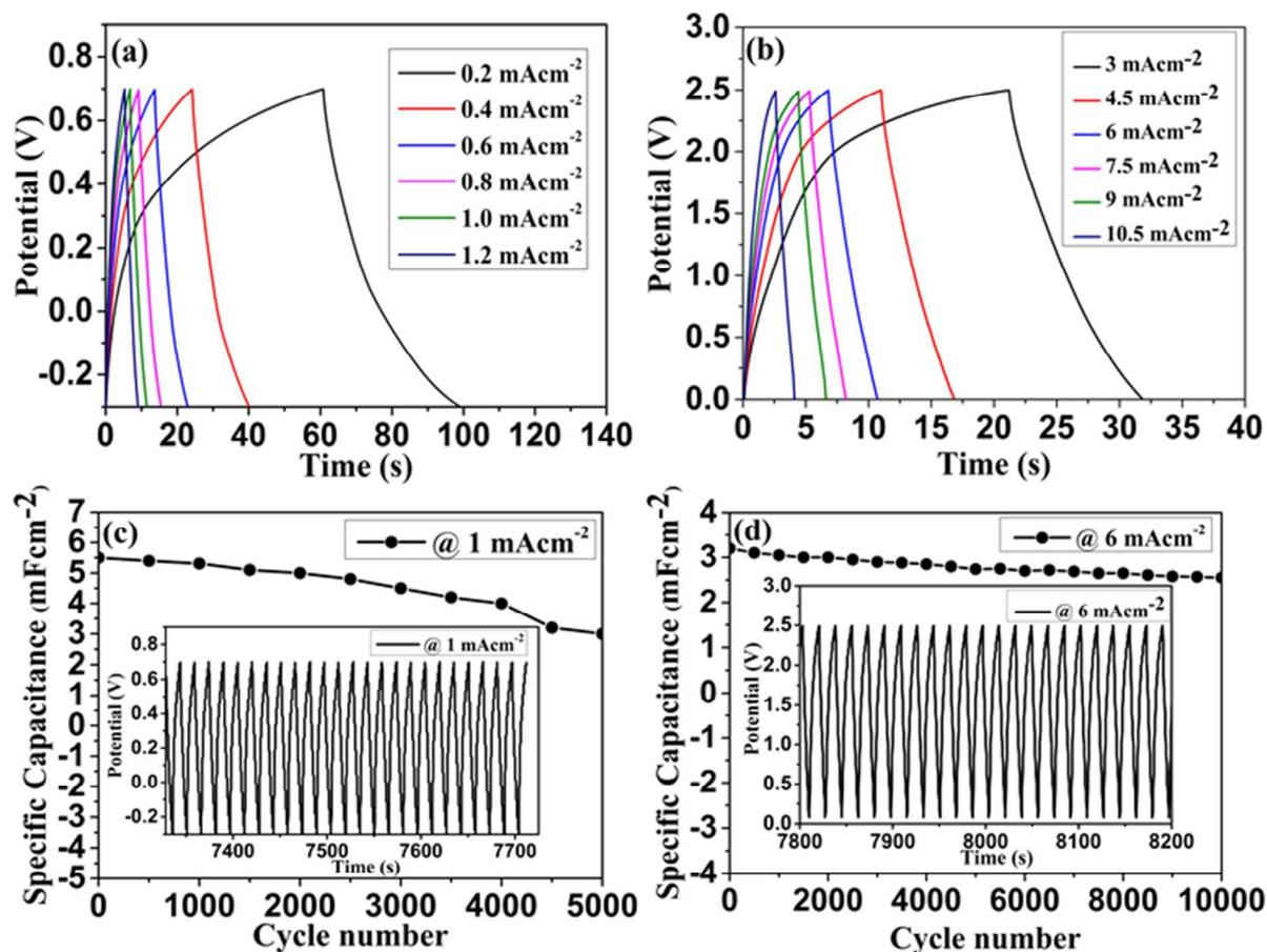
Figure 6. Charge-discharge profile of  $\text{Co}_3\text{O}_4/\text{CFC}$  based symmetric supercapacitor in 3 M KOH (a), 1 M TEABF<sub>4</sub> (b) and their corresponding cyclic performance (c & d).
