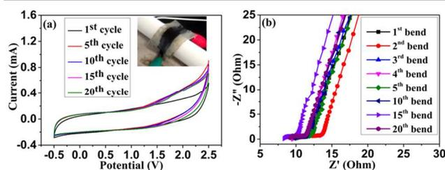
Figure 8. CV curves measured with bending position in organic electrolyte at 500 mVs<sup>-1</sup> (a) and Nyquist plot for the device measured at repeated bending (b).
