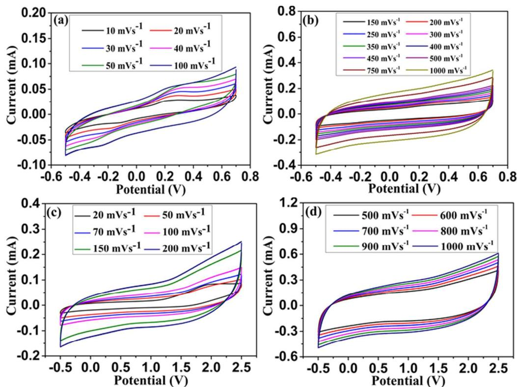
Figure 5. Cyclic voltammograms of  $\text{Co}_3\text{O}_4$  based symmetric supercapacitor in 3M KOH (a & b) and 1 M TEABF<sub>4</sub> in PC (c & d) measured at different scan rates.
