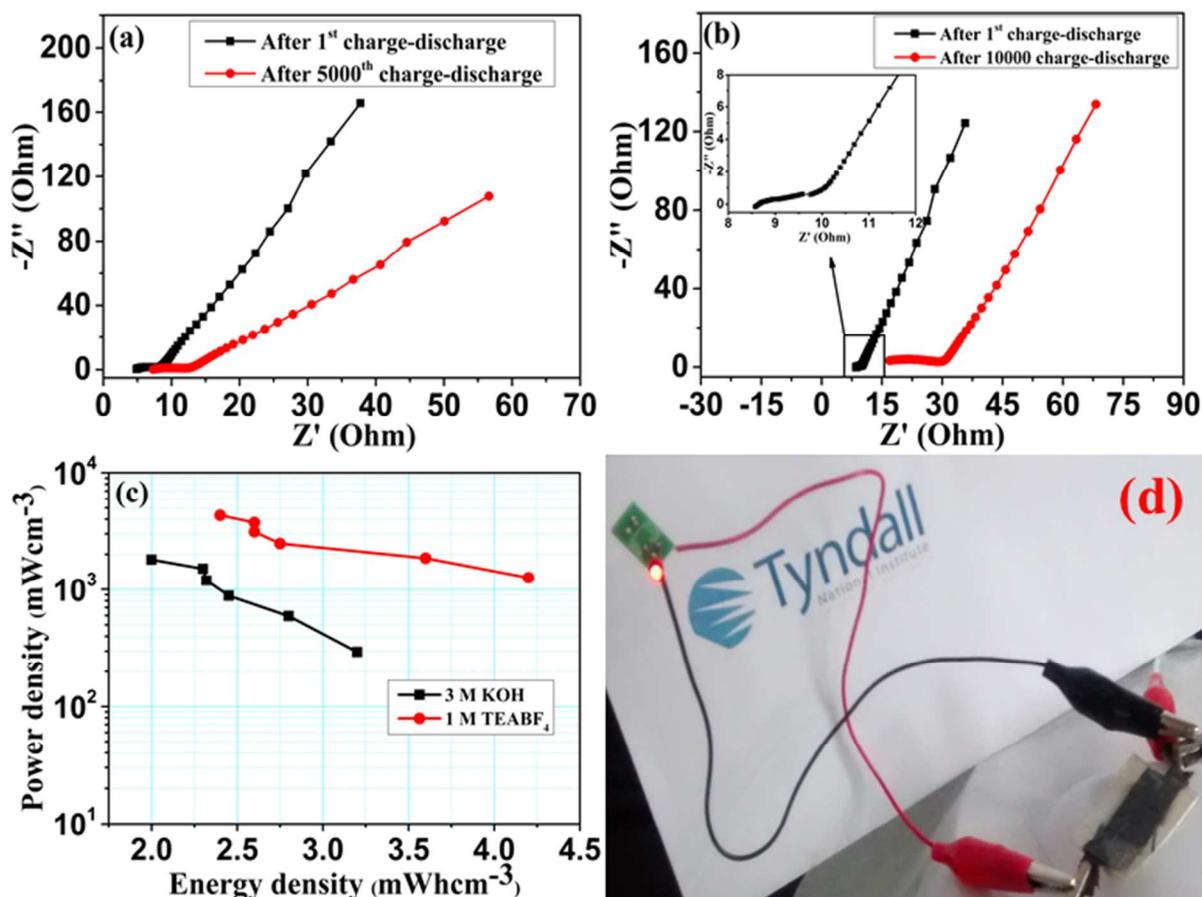
Figure 7. Nyquist plot of fabricated symmetric supercapacitor in (a) 3 M KOH, (b) 1 M TEABF<sub>4</sub>, (c) Ragone plots (Energy vs. Power) for the device in 3 M KOH (Black) and 1 M TEABF<sub>4</sub> (Red). (d) Optical photograph of a commercialized LED lighted by charged supercapacitor in 1 M TEABF<sub>4</sub>.
