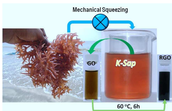
Figure 1. Reduction of graphene oxide in the presence of the seaweed sap extracted from Kappaphycus alvarezii .
