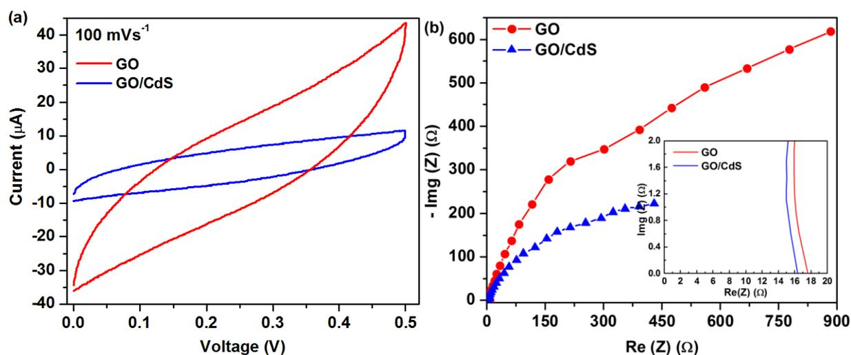
Fig. 10 (a) CV curves for GO sheet and GO/CdS nanocomposites working electrodes in 0.1 M Na<sub>2</sub>SO<sub>4</sub> electrolytes tested at a scan rate of 100 mV/s and (b) Nyquist plot for GO sheet and GO/CdS nanocomposites and the inset shows the enlarged view.
