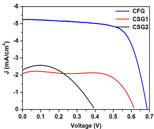
Simple surface functionalization of GO was employed with the quantum confined CdS towards the fabrication of *pn* hetero-junction based solar cell.
