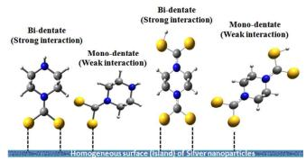
Fig. 9: Schematic demonstrations of possible interactions between adsorbates and silver islands (AgNPs).
