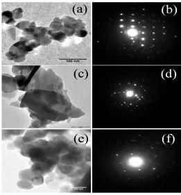
Fig.[ES2]: TEM images of (a) ZnONPs, (c) [PZCDT+ZnO], (e) [PZbCDT+ZnO], and SEAD images of (b) ZnONPs (d) [PZCDT+ZnO], 50 (f) [PZbCDT+ZnO]
