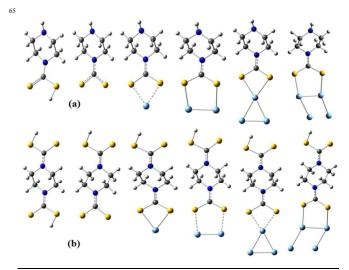
Fig. 2: (a) Optimized structures of PZCDT, deprotonated PZCDT, and PZCDT+ $Ag_{n=1,\,2,\,3,\,4}$ , (b) Optimized structures of PZbCDT, deprotonated PZbCDT, and PZbCDT+ $Ag_{n=1,\,2,\,3,\,4}$ ,
