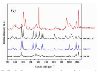
s Fig.[4]: Baseline corrected experimental normal Raman and SERS@ZnONPs spectra of PZCDT and PZbCDT in region (a) 3200 - 2650 cm<sup>-1</sup>, (b) 1730 - 1150 cm<sup>-1</sup> and (c) 1160 - 200 cm<sup>-1</sup>.
