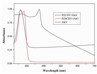
Fig.[5]: UV-Visible spectra of ZnONPs and complexes [ZnONPs + PZCDT/PZbCDT].
