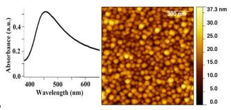
Fig 8: UV-Visible spectra and AFM image of as synthesized Ag island film
