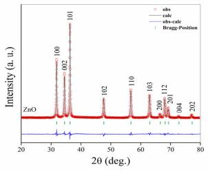
10 Fig ES1: XRD pattern of synthesized ZnO nanoparticles.
