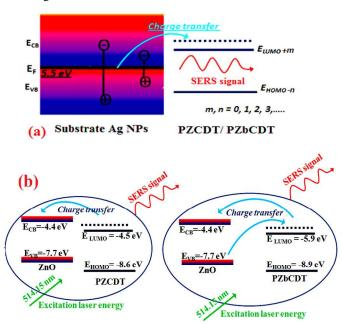
50 Fig.[6]: Schematic representation of suggested charge transfer mechanism in (a) SERS@AgNPs and (b) SERS@ZnONPs.
