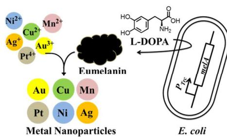
This study used the recombinant *E. coli* strain expressing the biomolecule, eumelanin, as an agent for the reduction of metal ions.
