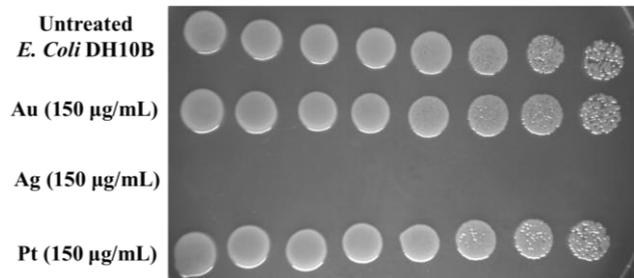
**Fig. 3** Growth and comparison of various metal nanoparticles treated cells. Quantitative survival measurements of *E. coli* DH10B in the presence or absence of 150 $\mu$ g/mL of Au, Ag, or Pt nanoparticles.
