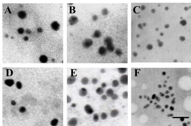
**Fig. 2** TEM images of diverse metal nanoparticles synthesized by recombinant *E. coli*. 100nM IPTG and 1 mM L-DOPA were used to induce the expression of EuMel for 12 h. EuMel solution was incubated with the corresponding 2mM of metal ions. (A) Au, (B) Ag, (C) Cu, (D) Mn, (E) Pt, and (F) Ni. Scale bar : 50 nm.
