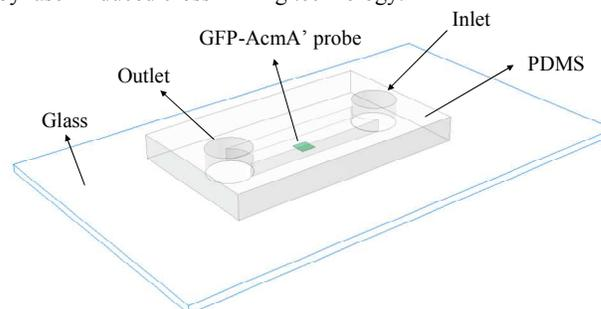
Fig. 6 3D schematic illustration showing microchannel design
