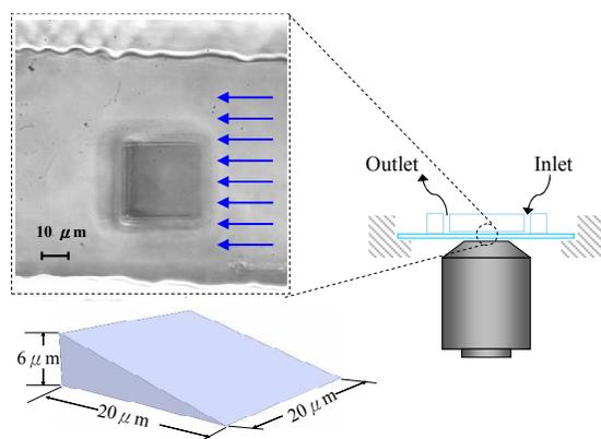
Fig. 7 Illustration of the laser-induced GFP-AcmA' probe in a microchannel and the dimension of the wedge-shaped probe
