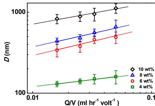
**Fig. 1** Plots of the relation between nanofiber diameter ( $D$ ) and flow rate divide by applied voltage ( $Q/V$ ) with respective to various concentrations of polymer blending solutions, i.e. 4 wt%, 6 wt% 8 wt% and 10 wt%. The samples are with polymer blending ratio of PU/EC = 1/1, i.e. P1C1.
