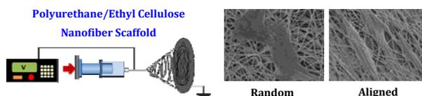
A high mechanical strength and biomimetic scaffold is fabricated by electrospinning a blend of polyurethane and ethyl cellulose. The scaffold with aligned fibers shows high biocompatibility with spindle cell morphology similar to nature tissues. This developed scaffold promises the application in therapeutic purposes of cardiac graft for reconstructing or regeneration of damaged myocardium.
