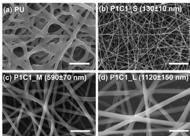
**Fig. 2** SEM images of PU and PU/EC scaffolds with blending ratio of PU/EC = 1/1 with various nanofiber diameters, i.e. (a) PU, (b) P1C1\_S, (c) P1C1\_M, and (d) P1C1\_L. The average diameters and standard deviations were calculated from over 20 measured widths of the nanofibers in the SEM images. The scale bar is 50  $\mu\text{m}$  in length.
