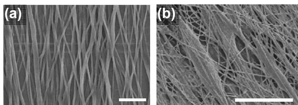
**Fig. 6** (a) SEM image of PU/EC scaffold (ratio of 9/1) with aligned nanofibers, i.e. P9C1\_L\_A. (b) SEM image of P9C1\_L\_A scaffold after H9C2 cells cultured for 4 hrs. The scale bar is 100  $\mu\text{m}$  in length.
