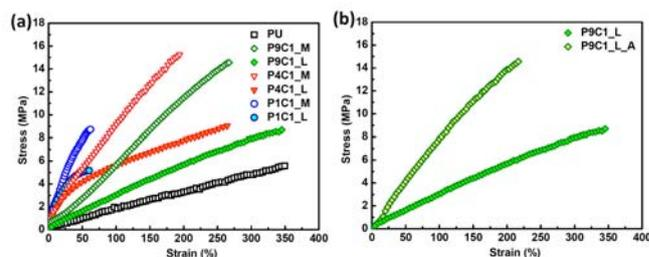
**Fig. 5** (a) Stress-strain curves of pristine PU scaffolds and PU/EC scaffolds with different nanofiber diameters with respect to different blending ratios, *i.e.* P9C1\_M, P9C1\_L, P4C1\_M, P4C1\_L, P1C1\_M, and P1C1\_L. (b) Stress-strain curves of PU/EC (ratio of 9/1) scaffolds with isotropic and aligned nanofibers ( $\sim$ 1000 nm), *i.e.* P9C1\_L and P9C1\_L\_A respectively.
