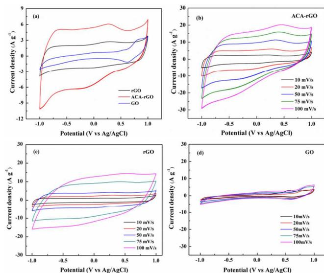
**Fig 7** (a) CV curves of ACA-rGO, rGO, and GO at the scan rate 20 mVs<sup>-1</sup> and CV curves of (b) ACA-rGO, (c) rGO, and (d) GO at scan rates of 10, 20, 50, 75, and 100 mV s<sup>-1</sup>.
