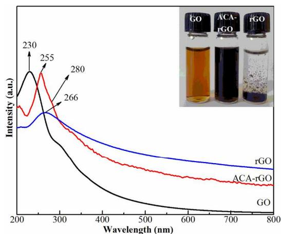
Fig. 2 UV-vis spectra of GO, ACA-rGO and rGO.
