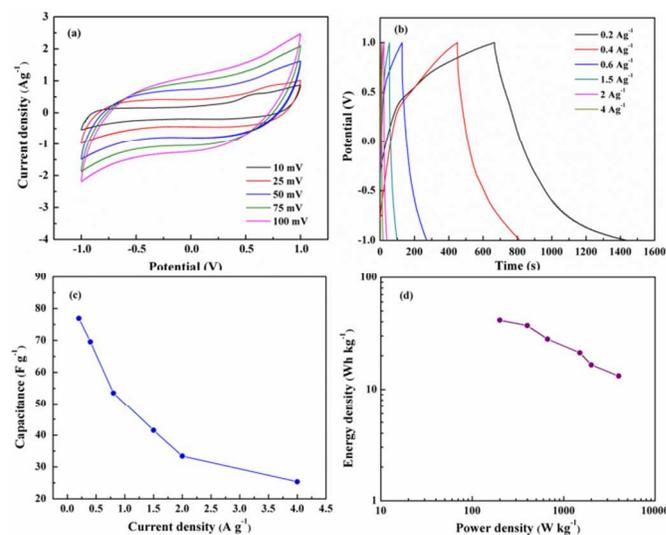
**Fig. 10** (a) CV curves of asymmetric cell with ACA-rGO and CNT, (b) galvanometric charge-discharge curves, (c) cell capacitance value with different current density, and (d) Ragone plot of two electrode cell.
