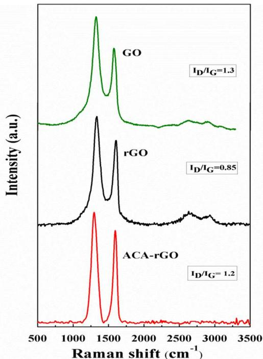
Fig 4 Raman spectra of GO, rGO and ACA-rGO
