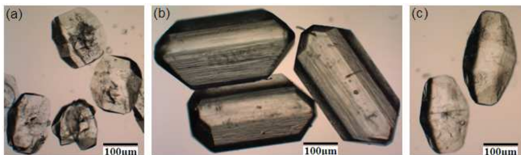
Fig. 2 Optical microscopy images of \alpha -HNIW (a), cocrystal hydrate (b), and \varepsilon -HNIW (c)
