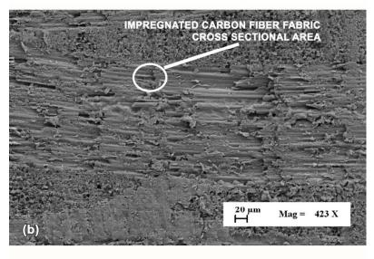
Fig. 8. SEM images, at two different magnification, of the cross sectional area of the manufactured panel.
