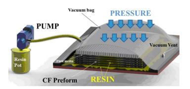
Fig. 1. Scheme of liquid resin infusion technique.
