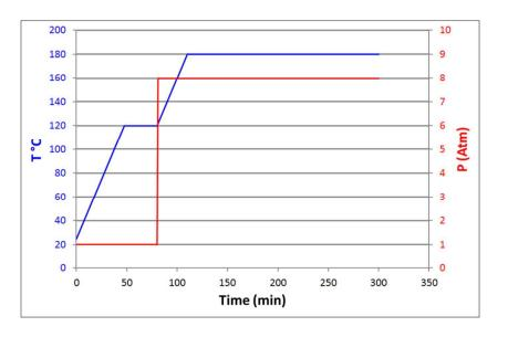
Fig. 6. Curing cycle and pressure for the Impregnation process.
