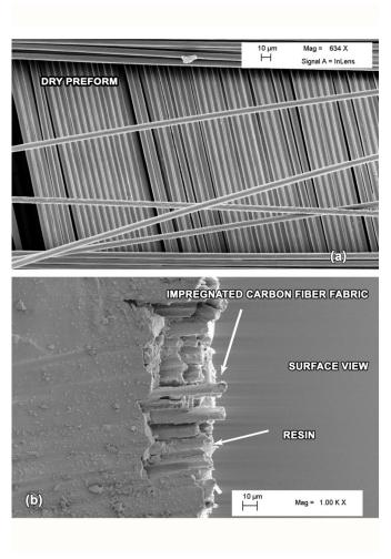
Fig. 9. FESEM image of the dry perform (a) and of the top side of the CFRC surface (b).
