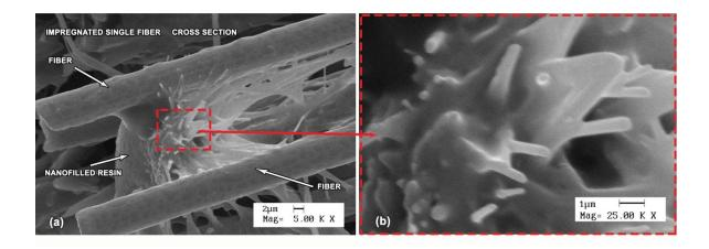
**Fig. 11.** SEM micrograph of carbon nanotubes in the resin impregnating the CFs and in the narrow matrix-rich regions between the fibers (a), detail of the presence of carbon nanotubes in the epoxy matrix (b).
