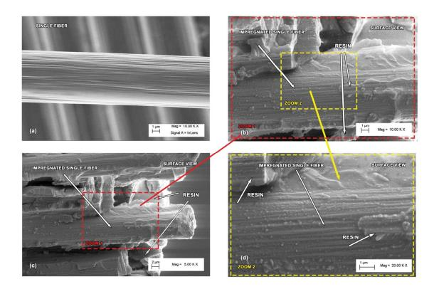
**Fig. 10.** SEM micrographs of single carbon fiber (a); detail at different magnification (b), (c) (d) of a single CF impregnated by the nanofilled resin.
