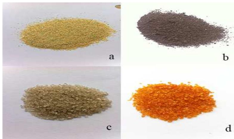
Fig. 2 Photographs of aTEPRs, bTEPRs and the sulfonated products of S-aTEPRs and S-bTEPRs. (a) aTEPRs, (b) S-aTEPRs, (c) bTEPRs, (d) S-bTEPRs.
