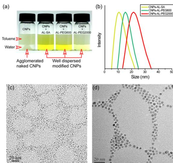
**Fig. 1** (a) CNPs surface coating using alendronate as anchor. (b) The hydrodynamic size distribution of surface coated CNPs. The TEM images of CNPs-AL-PEG600 synthesized by microemulsion (c) and high temperature decomposition method (d) dispersed in water.
