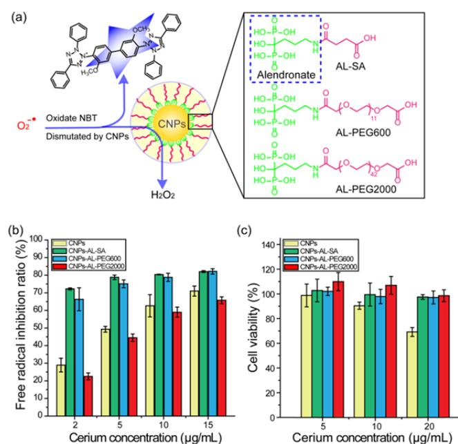
**Fig. 3** (a) Schematic illustration of the dismutation of superoxide free radical by surface coated CNPs, the free superoxide free radical reacted with nitro-tetrazolium blue chloride (NBT) to generate blue product which could be detected at 560 nm. (b) The superoxide free radical inhibition ratio of CNPs before and after surface coating. (c) The cell viability of CNPs before and after surface coating.
