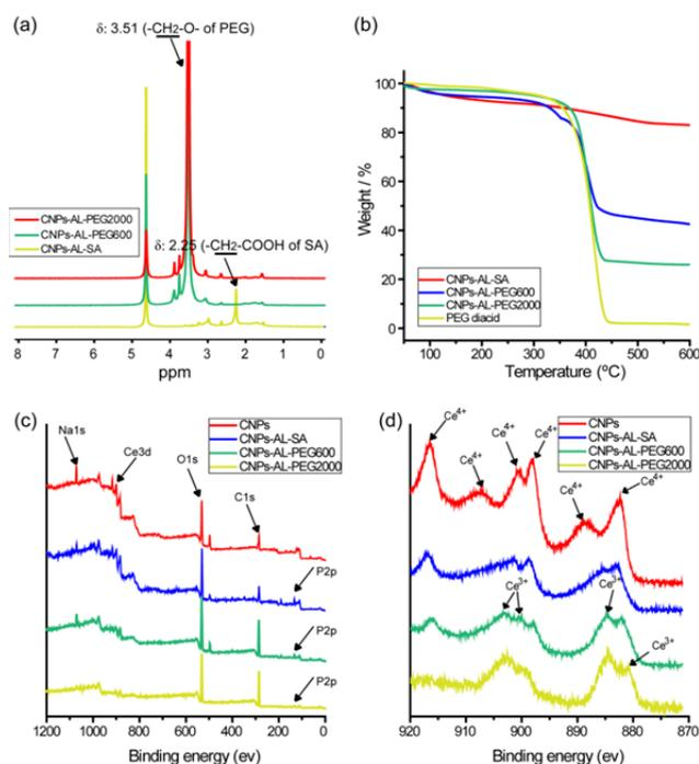
**Fig. 2** (a) The NMR spectra of surface coated CNPs. (b) the TGA graphs of surface coated CNPs. (c) The full XPS spectra of CNPs before and after surface coating. (d) Selected XPS segments related to valence state of cerium ions with corresponding binding energy peaks for  $\text{Ce}^{3+}$  (880.20, 885.00, 899.50 and 903.50 eV) and  $\text{Ce}^{4+}$  (882.10, 888.10, 898.00, 900.90, 906.40 and 916.35 eV).
