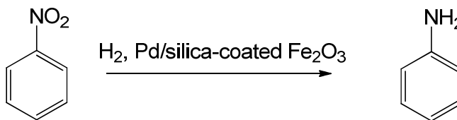
Scheme 22. Catalytic hydrogenation of nitrobenzene to aniline.
