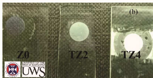
Fig 4 (a) Diffuse reflectance spectra of the Z0 and TZ1 to TZ5 films (b) Digital image of identical samples on ITO substrate
