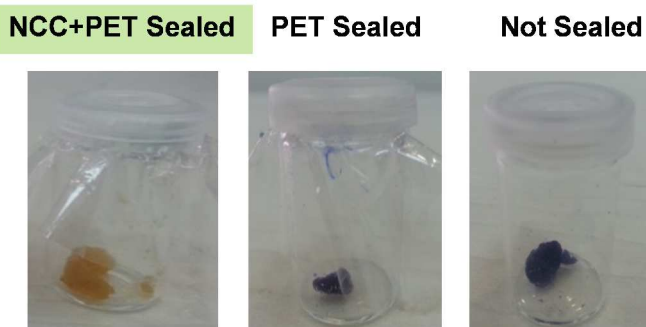
Fig. 6 Oxidation experiment with the color dye of methylene blue after 24 hours under room conditions with pierced caps. The methylene blue gel remained un-oxidized when covered with PET+NCC. When covered with PET or not covered the methylene blue oxidized.
