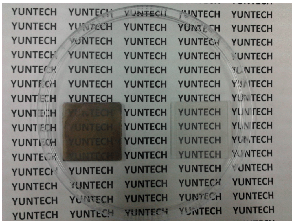
Fig. 6. Photographs of AgNW (left) and 3.2 wt.% PES-AgNW (right) electrodes exposed to air at room temperature over 15 days.
