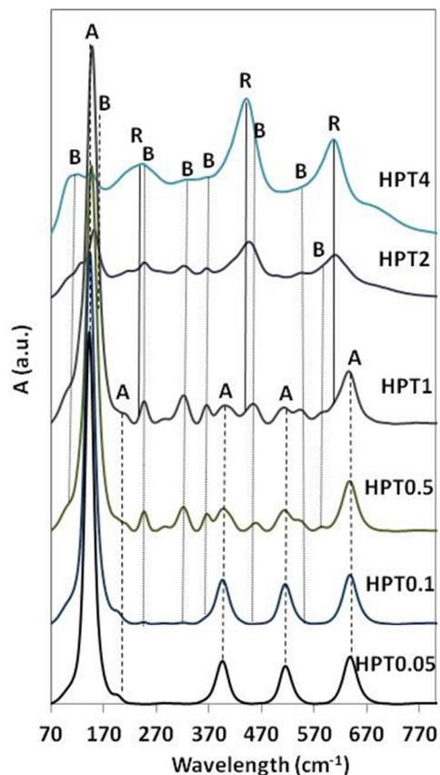
Figure 3. Raman spectra of HPT TiO<sub>2</sub> samples. A, B and R are referring to the representative vibrations of anatase, brookite, rutile, respectively.
