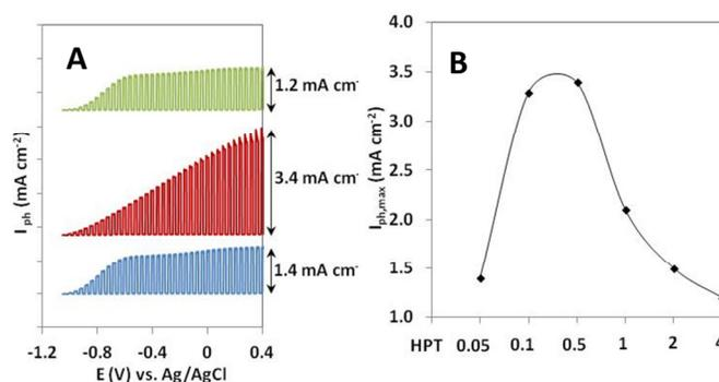
Figure 5 A). Representative photo-voltammograms of selected TiO<sub>2</sub> samples, recorded between -1.1 V and 0.5 V, in 0.1 M Na<sub>2</sub>SO<sub>3</sub>, at a sweep rate of 2 mV s<sup>-1</sup> using a 300W Hg-Xe arc lamp. B) Comparison of the maximum photocurrent values obtained for the various TiO<sub>2</sub> samples.
