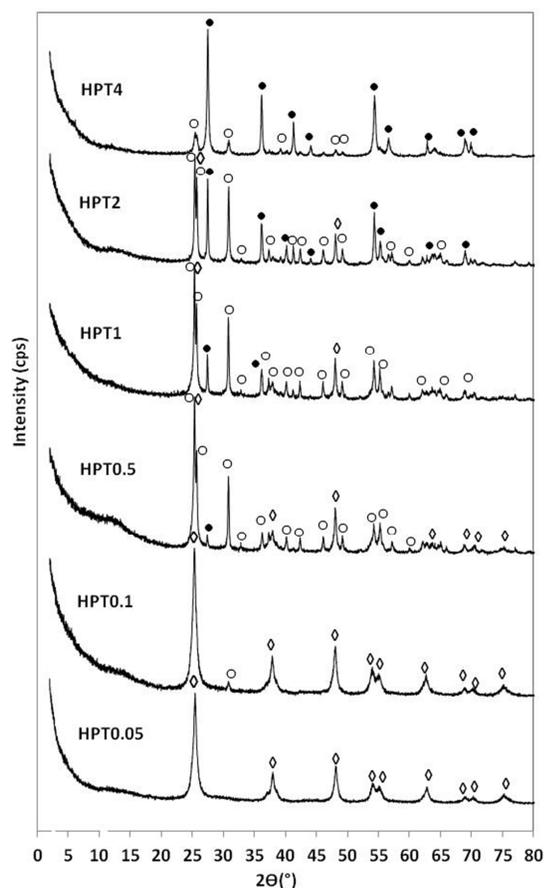
Figure 1. XRD patterns of HPT  $\text{TiO}_2$  samples:  $\diamond$  Anatase;  $\circ$  Brookite;  $\bullet$  Rutile
