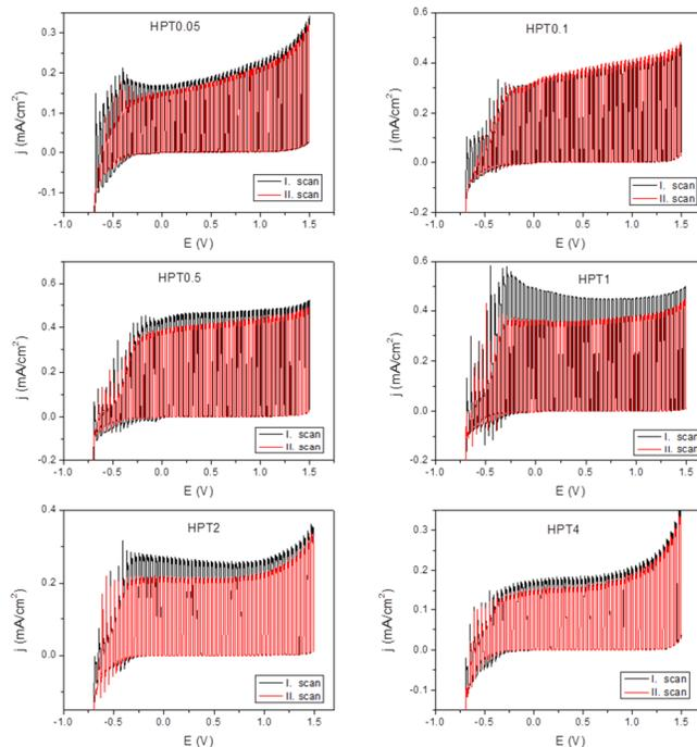
**Figure 6.** Different decaying behaviours of the photocurrents of the TiO<sub>2</sub> samples assessed by consecutive photovoltammometric scans. The scans were recorded between -0.7 V and 1.5 V, in 0.1 M Na<sub>2</sub>SO<sub>4</sub>, at a sweep rate of 2 mV s<sup>-1</sup> using a 300W Hg-Xe arc lamp.
