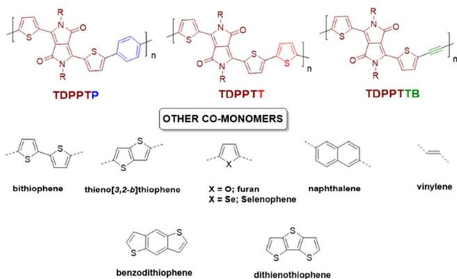
**Scheme 1** Chemical structures of the various DPP alternating copolymers
