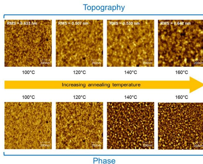
**Fig. 4** AFM measurements showing topography and phase images of TDPPTTB film annealed at different temperatures. The scan size is 1  $\mu\text{m}$  by 1  $\mu\text{m}$ .
