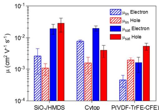
**Fig. 7** Mobilities ( $\mu$ ) of TDPPTTB transistors based on different dielectrics. All values are calculated from  $120 \text{ }^\circ\text{C}$ -annealed TDPPTTB films.
