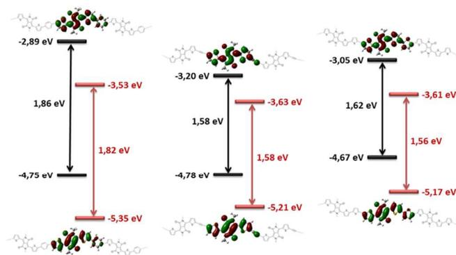
**Fig. 3** Calculated HOMOs and LUMOs of the tetramer model compounds of the polymers using DFT at B3LYP/6-31(d,p) level of theory (black lines) and experimental energy levels obtained by cyclic voltammetry measurements (red lines) of TDPPTP (left), TDPPTB (center), and TDPPTTB (right)
