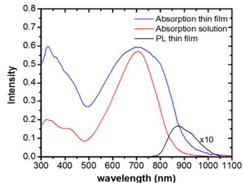
**Fig. 2** Absorption spectra of TDPPTTB in chloroform solution and as thin film
