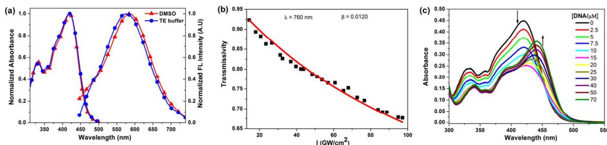
Fig. 1 (a) Normalized absorption and one-photon induced fluorescence spectra of **BMEPC** in DMSO and TE buffer; (b) The plot of transmissivity dependence on light intensity for **BMEPC** at 760 nm. Squares denote the experimental value of transmissivity; solid lines denote the theoretical fitting line; (c) The absorption spectra of **BMEPC** (10  $\mu\text{M}$ ) with the addition of CT-DNA (0-70  $\mu\text{M}$ ) in TE buffer.
