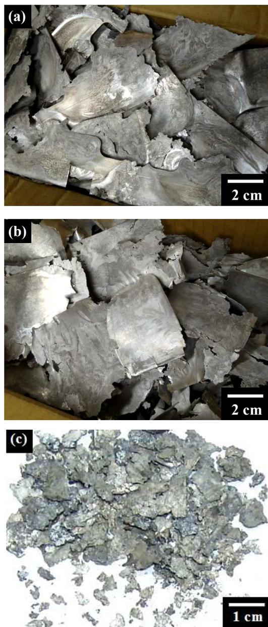
**Fig. 3** Mg alloys die casting flash scraps that currently can not be recycled economically: (a) AM60 scrap; (b) AZ91 scrap. The thin flash scraps easily to be broken down to small pieces, as shown in (c).
