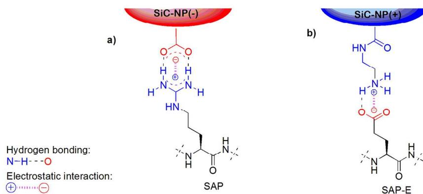
**Figure 2.** Expected non-covalent interactions between oppositely charged SiC-NPs and CPPs. As-prepared anionic SiC-NP(-) interacting with arginine side chains of SAP (a); and cationic SiC-NP(+) interacting with glutamate residues of SAP-E (b).
