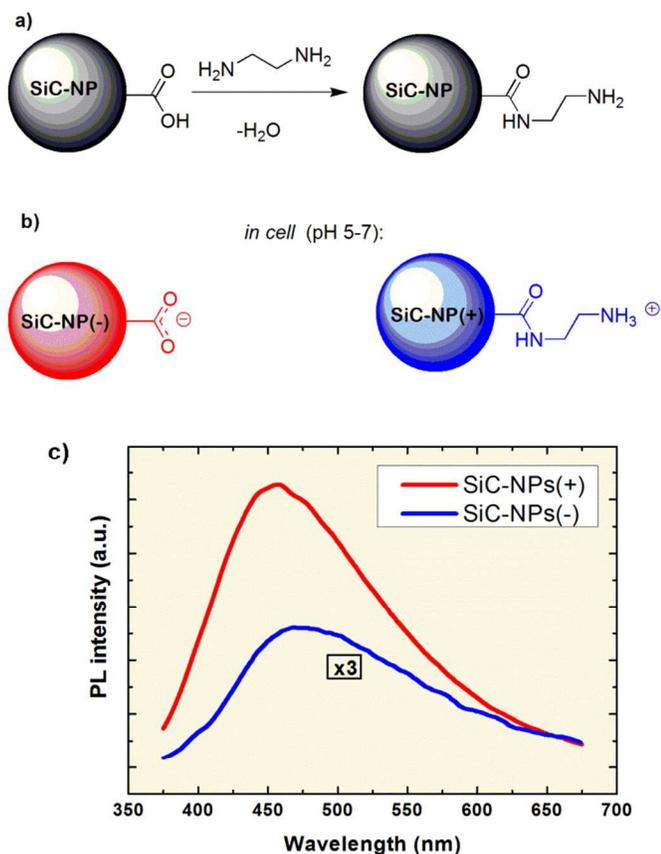
**Figure 1.** Chemical modification of the carboxylic groups on the surface of the SiC-NPs (a), their ionization states under cellular internalization conditions (b), and photoluminescence spectra (excitation at 343 nm) of the as-prepared SiC-NPs used in this study (c).
