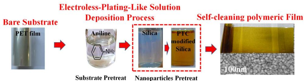
**Scheme 1** Scheme of electroless-plating-like solution deposition (EPLSD) process for fabricating the TiO<sub>2</sub>-SiO<sub>2</sub> self-cleaning polymeric film.
