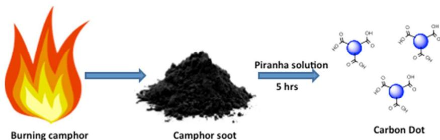
**Fig. 1** Illustration of the formation of C dots from thermal dissociation of camphor
