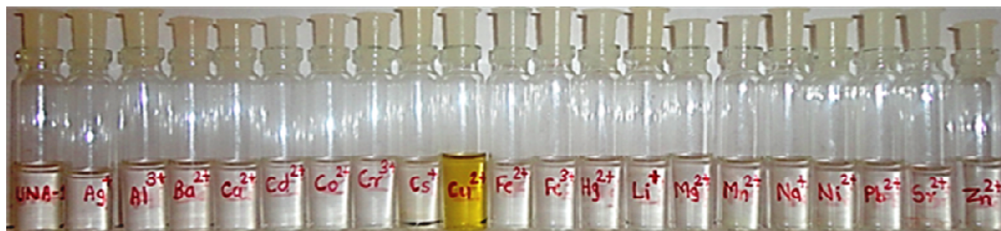
Fig. 1. Naked-eye detectable color change of ions with UNA-1 in the presence of 5 equivalents of different cations.
