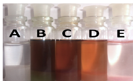
Fig. 9. UNA-1 supported silica gel was treated with different concentrations of \text{Cu}^{2+} . A=silica without UNA-1 + 1 \times 10^{-3} M \text{Cu}^{2+} as control.
