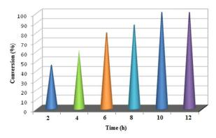
Fig. 9. Effect of reaction time on one pot three component coupling reaction (Reaction conditions: phenyl acetylene (1 mmol), dichloromethane (2 mmol), diethylamine (2 mmol), DBU (1 mmol), solvent (2 mL), catalyst (30 mg), temp. 70°C)
