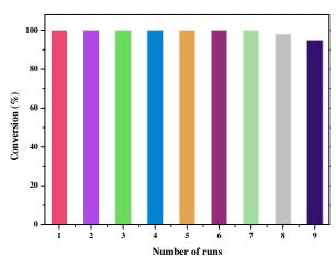
Fig. 10 Catalytic reusability test for one pot three component coupling reaction (reaction conditions: phenyl acetylene (1 mmol), dichloromethane (2 mmol), diethylamine (2 mmol), DBU (1 mmol), acetonitrile (2 mL), catalyst (30 mg), temp. 70°C, time 10 h)
