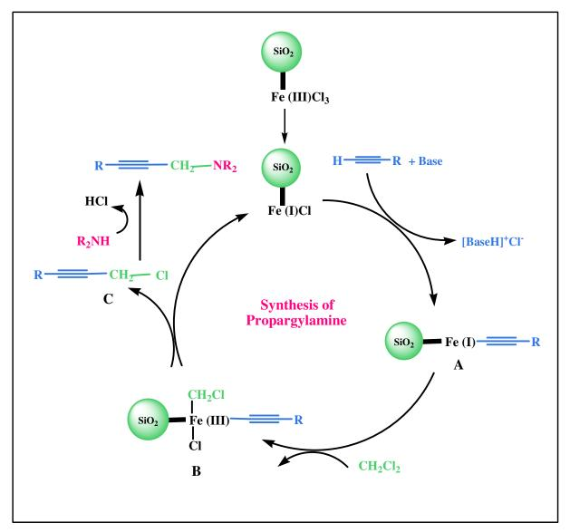
Scheme 2 Probable reaction mechanism of SiO<sub>2</sub>@ APTES@DAFO-Fe catalyzed one pot three component coupling of terminal alkynes, dichloromethane and secondary amines.
