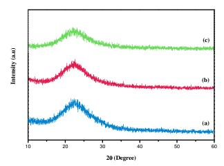
Fig. 2 XRD diffraction patterns of (a) SiO<sub>2</sub>, (b) SiO<sub>2</sub>@APTES and (c) SiO2@APTES@DAFO-Fe
