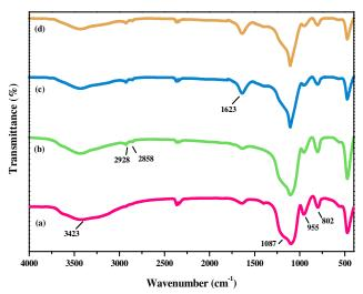
Fig. 1 FT-IR spectra of (a) SiO<sub>2</sub>, (b) SiO<sub>2</sub>@APTES and (c) SiO<sub>2</sub>@APTES@DAFO-Fe (d) recovered SiO<sub>2</sub>@APTES@DAFO-Fe
