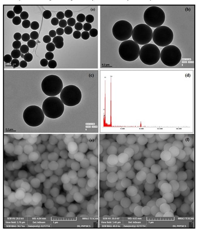
Fig. 3 TEM micrographs of (a) SiO<sub>2</sub> and (b) SiO<sub>2</sub>@APTES@DAFO-Fe. (c) Recovered SiO<sub>2</sub>@APTES@DAFO-Fe. (d) EDX spectrum of SiO<sub>2</sub>@APTES. (e) and SEM images of (e) SiO<sub>2</sub>@APTES@DAFO-Fe. (f) Recovered SiO<sub>2</sub>@APTES@DAFO-Fe.
