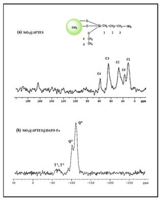
Fig. 4 (a) <sup>13</sup>C CPMAS NMR spectrum of SiO<sub>2</sub>@APTES and (b) <sup>29</sup>Si CPMAS NMR spectrum of SiO<sub>2</sub>@APTES@DAFO-Fe.
