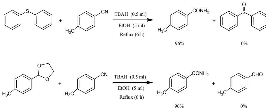
**Scheme 3.** Selective synthesis of 4-methylbenzamide using tetrabutylammonium hydroxide in the presence of 2-(4-methylphenyl)-1,3-oxazoline and diphenyl sulfide
