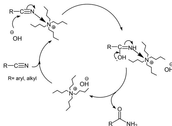
**Scheme 5.** Suggested mechanism for the hydrolysis of nitriles by hydrated ionic liquid (IL) tetrabutylammonium hydroxide.
